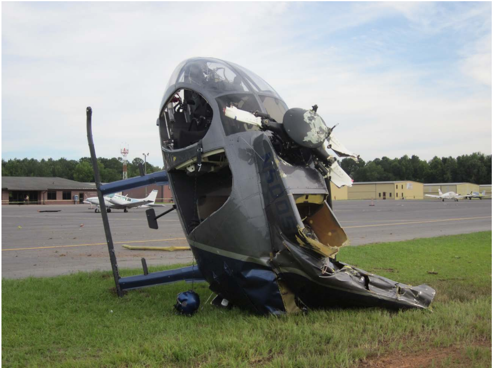
Photo 1 – View of helicopter damage to the main rotor system, fuselage, tailboom, and tail rotor system (courtesy of the FAA)
