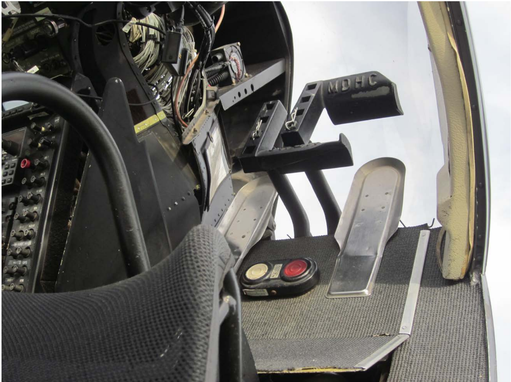
Photo 2 – View of right side tail rotor control pedals (courtesy of the FAA)
