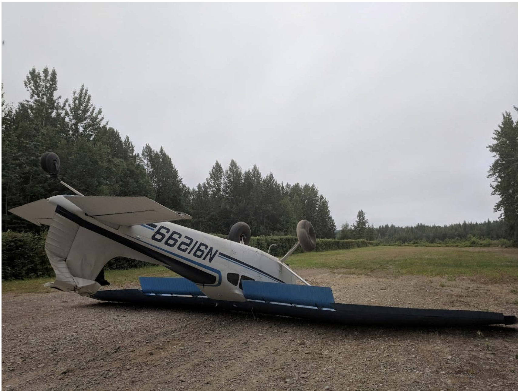
Photo 1 – View of inverted airplane and damaged empennage (Photo courtesy of the pilot)
