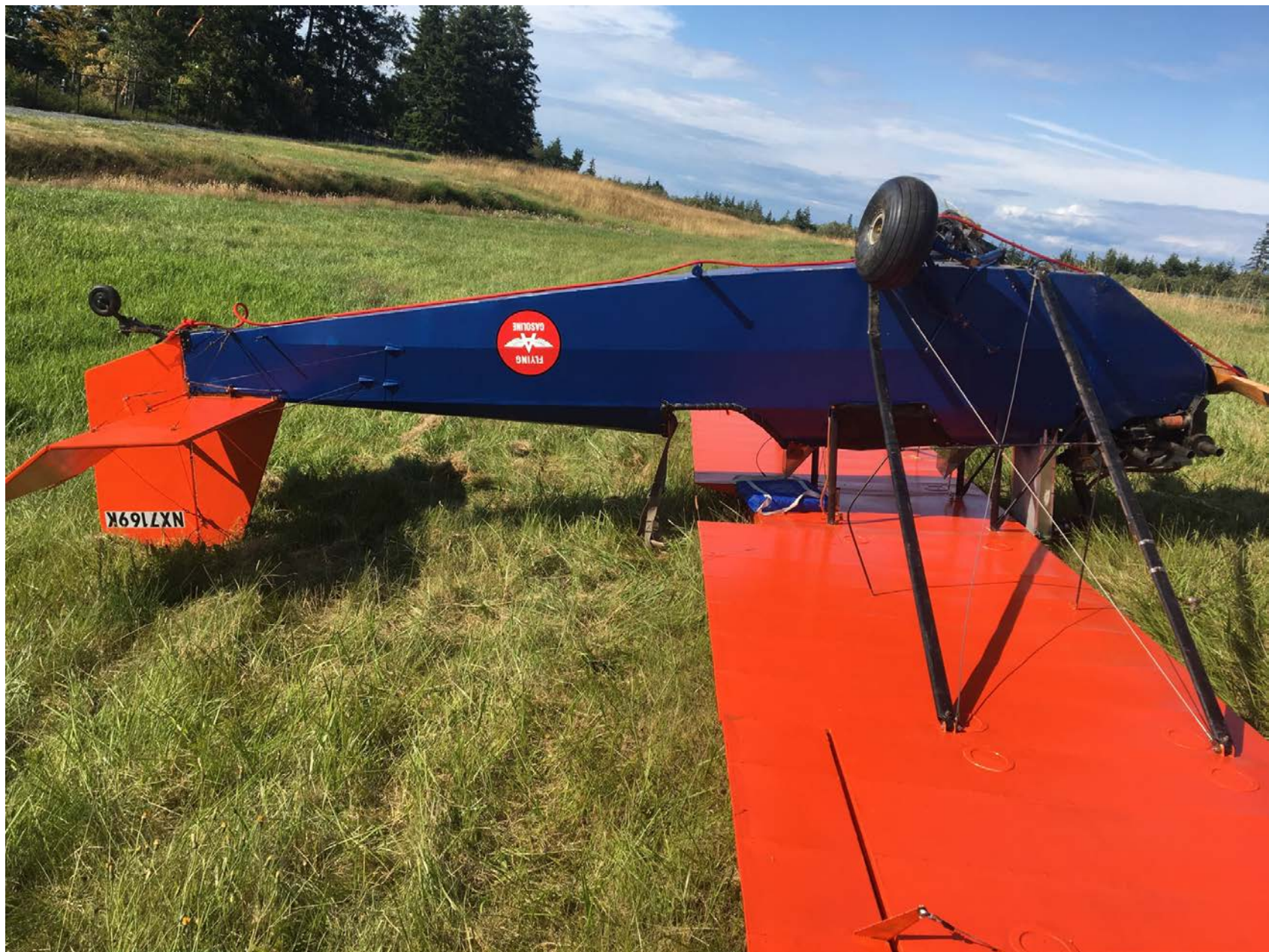
Photo 1 – View of damage to the left wing lift strut (Courtesy of Operator)
