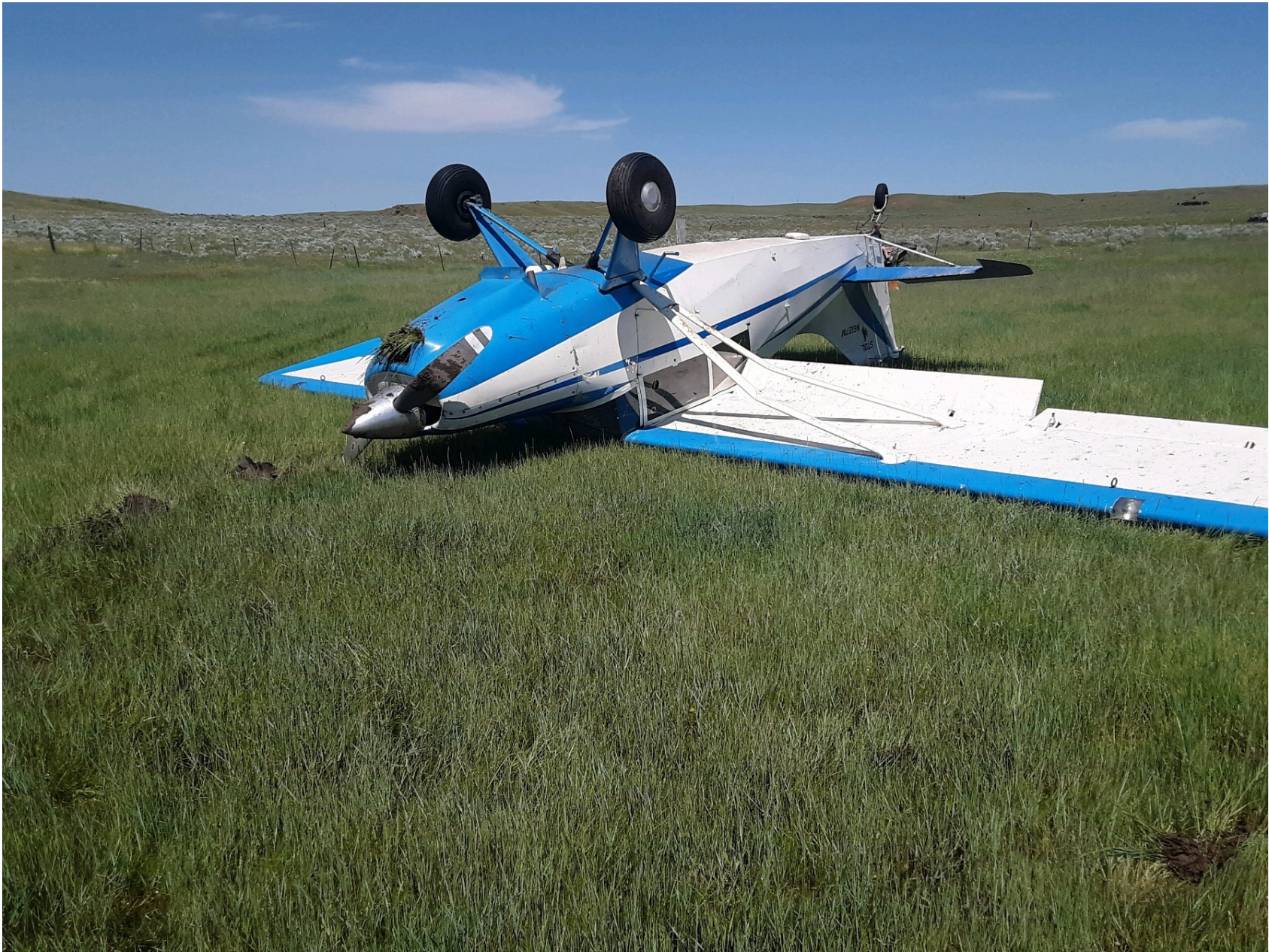
Photo 1 – View of damaged right-wing lift strut (courtesy of the pilot)
