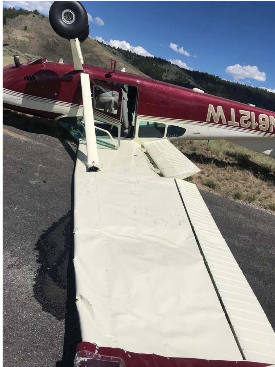
Photo 2 - View of right wing damage (photo courtesy of the FAA)
