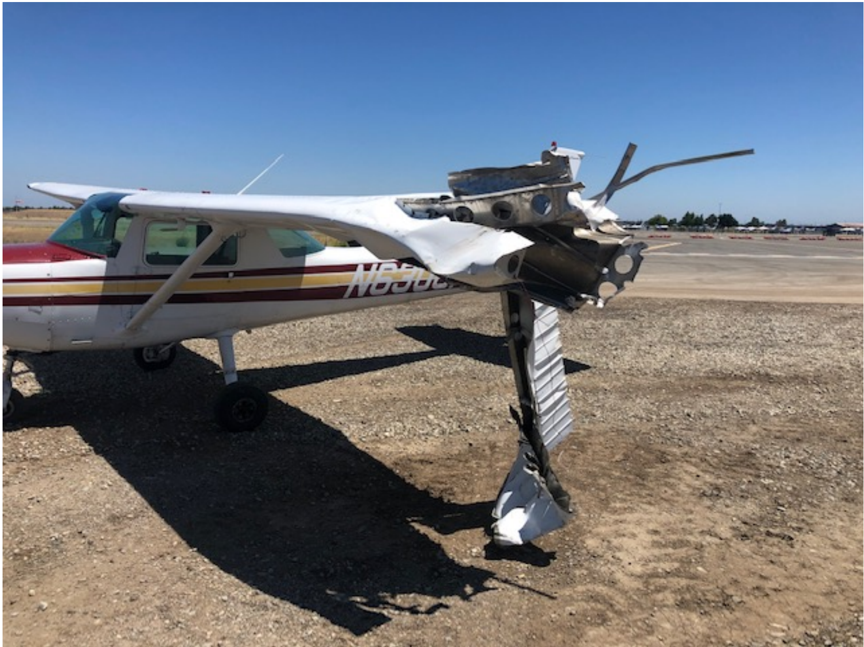
Photo 1 – View of damaged left wing (courtesy of the operator)
