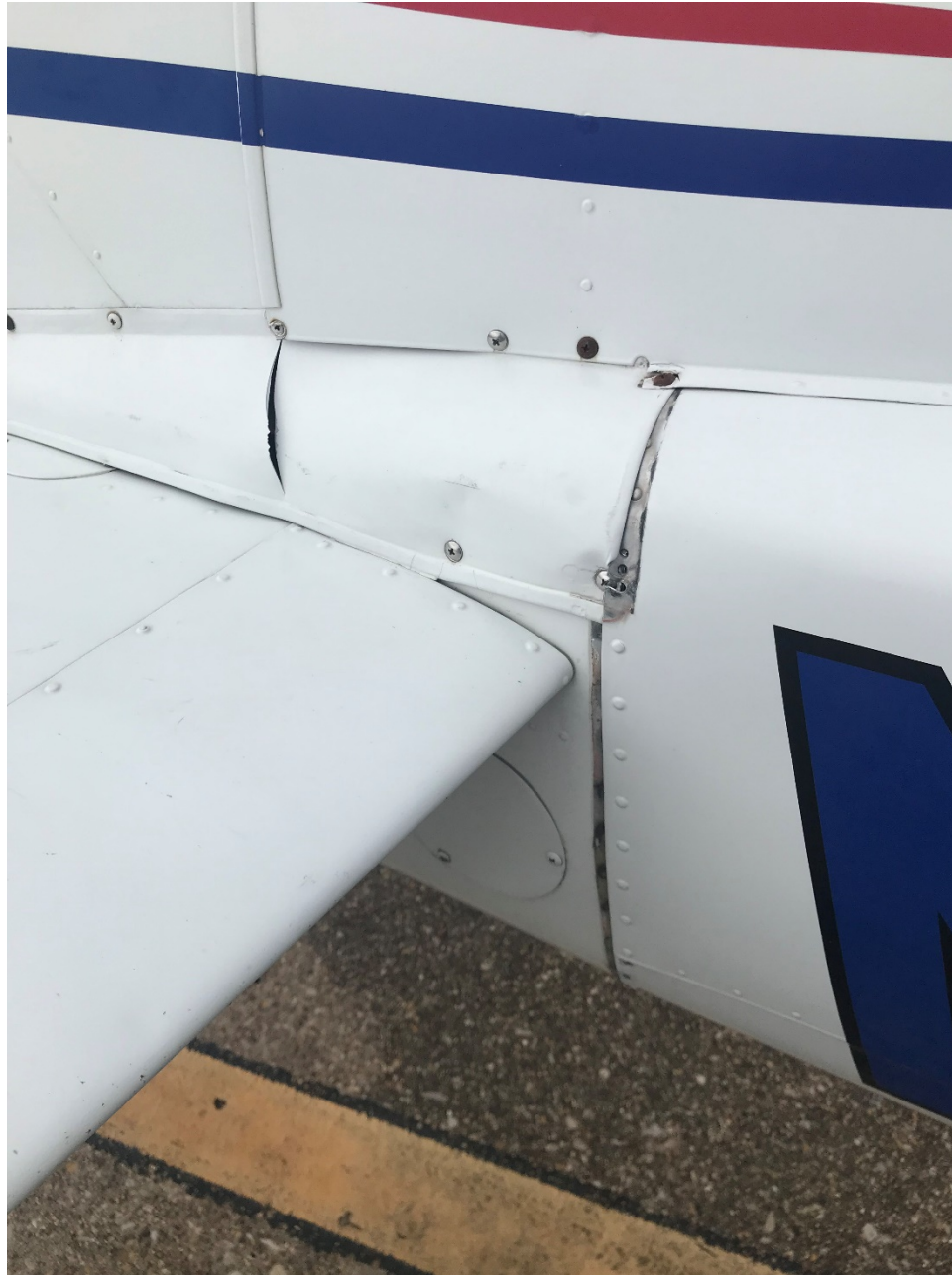
Photo 1 – View of empennage damage (Photo courtesy of the FAA)
