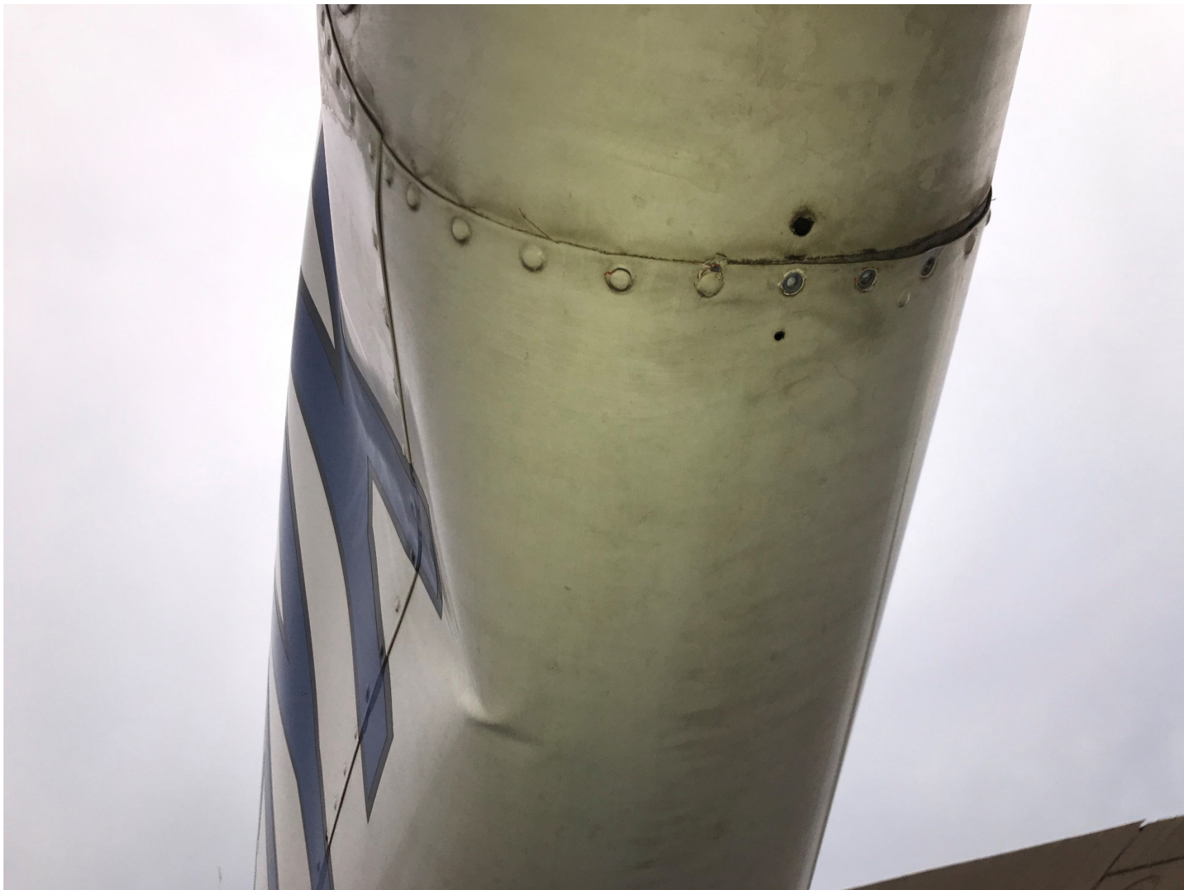
Photo 2 – View of fuselage damage from underneath (Photo courtesy of the FAA)
