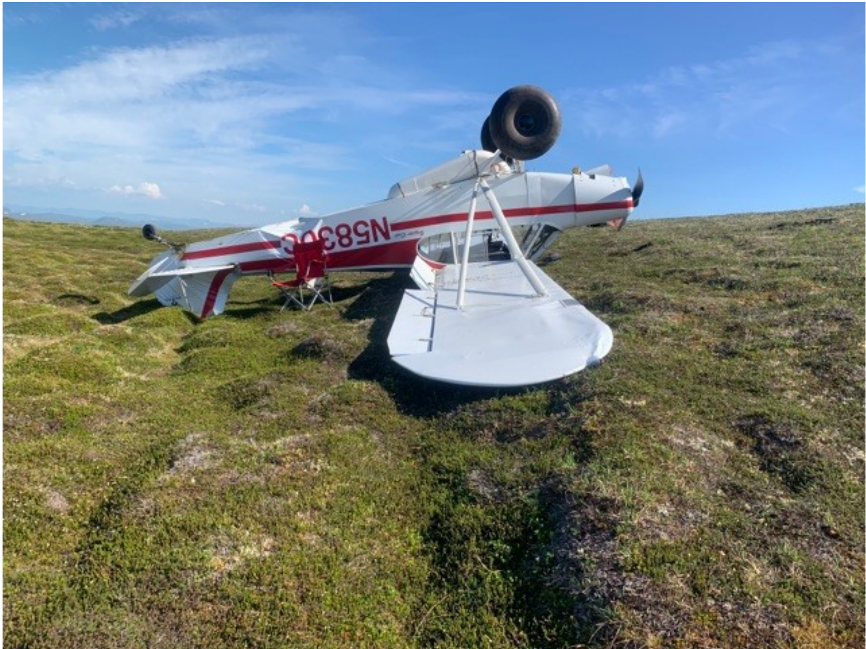
Photo 1 – View of fuselage and wing lift strut damage (photo courtesy of the FAA)
