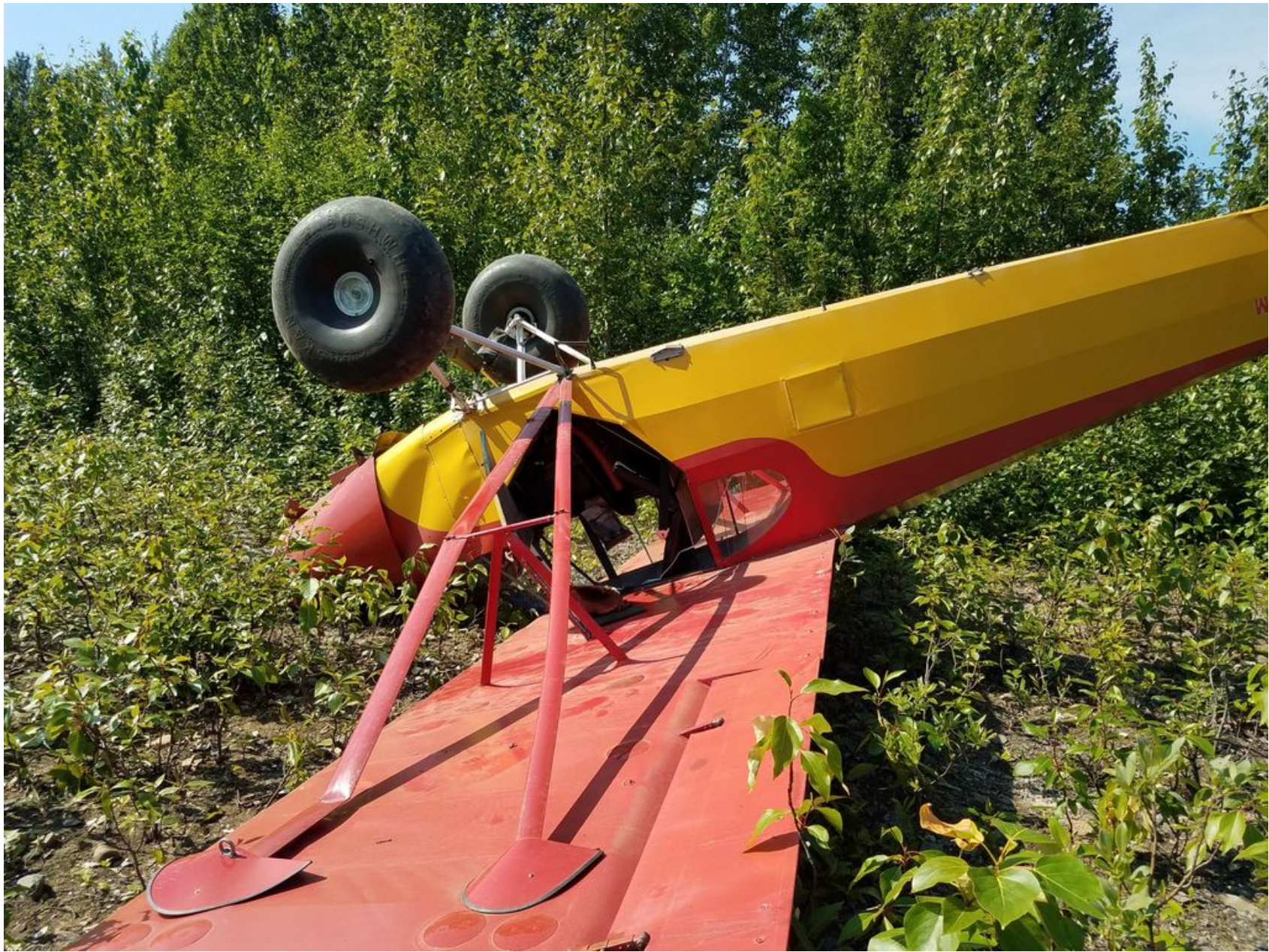
Photo 1 – View of damaged right-wing lift strut (courtesy of the FAA)
