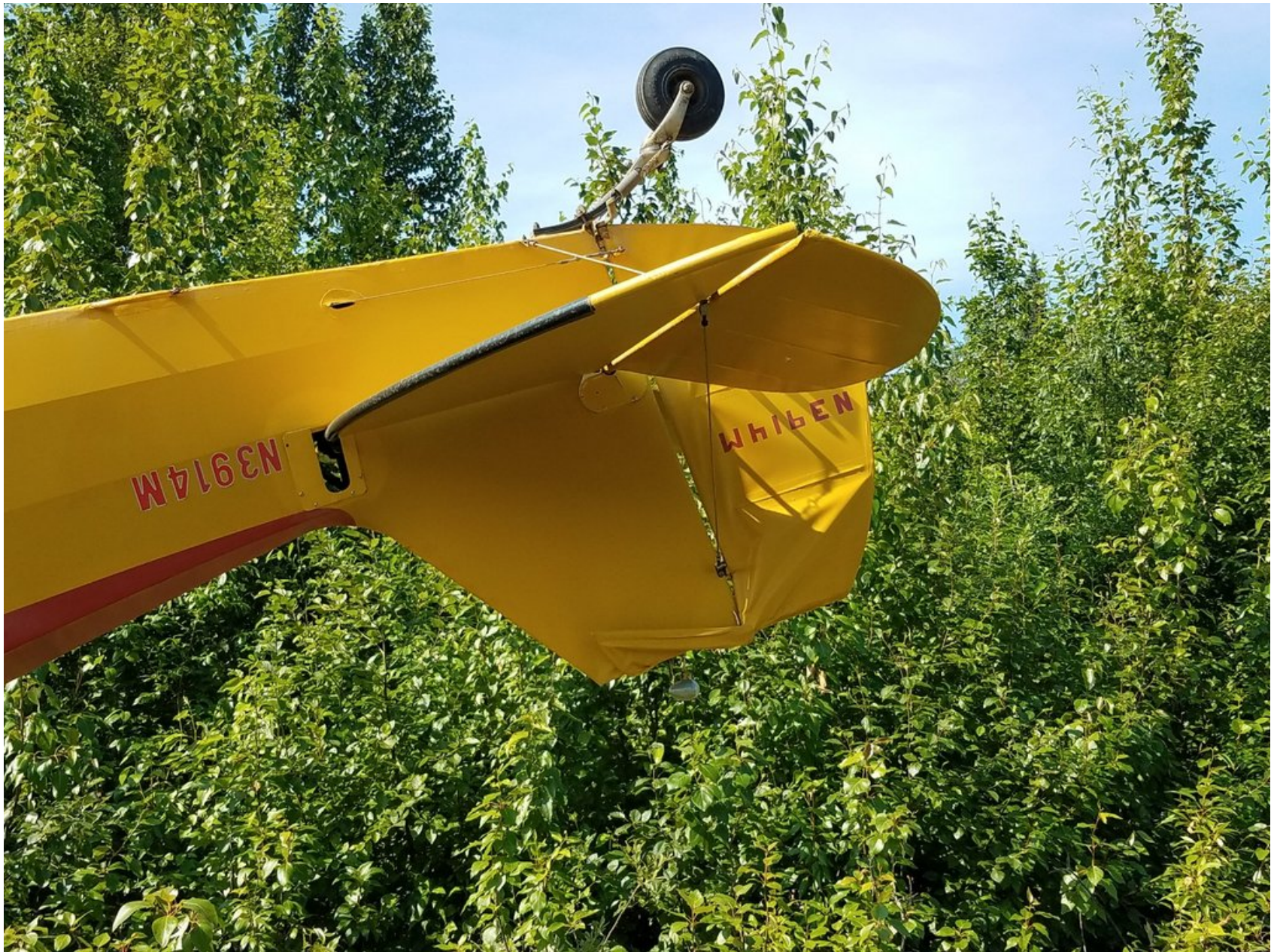
Photo 2 – View of damaged vertical stabilizer and rudder (courtesy of the FAA)
