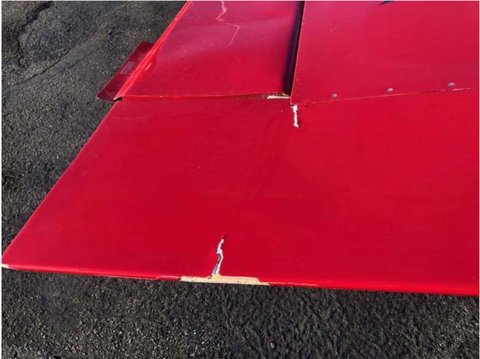
Photo 1 – View of right aileron damage (Photo courtesy unknown)
