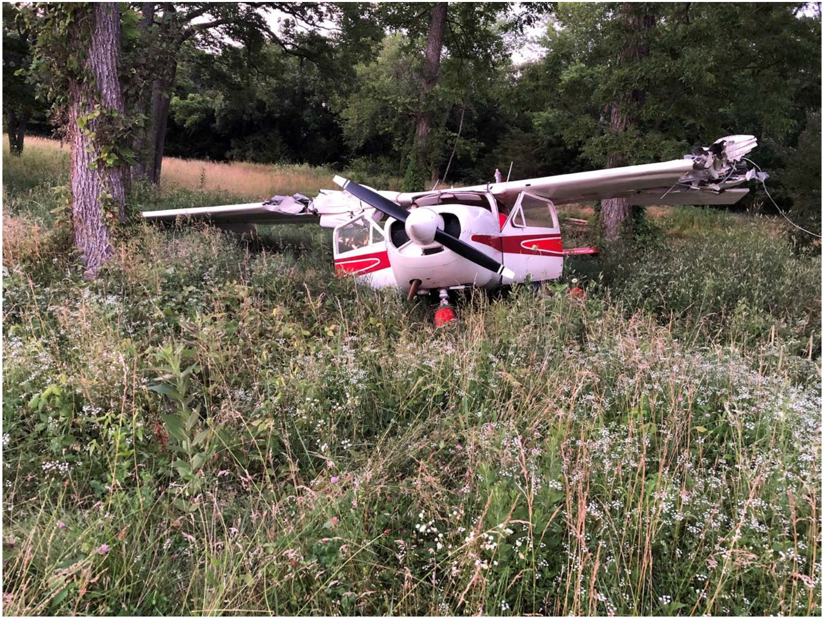
Photo 1 – View of damage to both wings (courtesy of the pilot)
