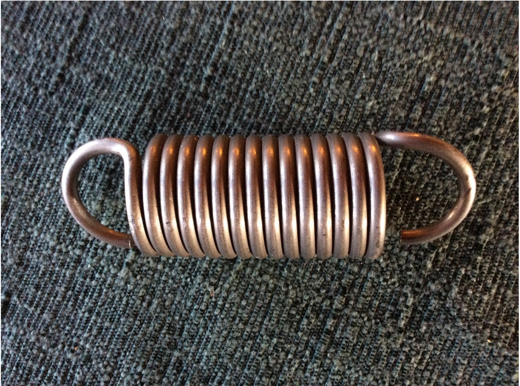
Photo 3 – View of left steering spring found on runway (Photo courtesy of the pilot)
