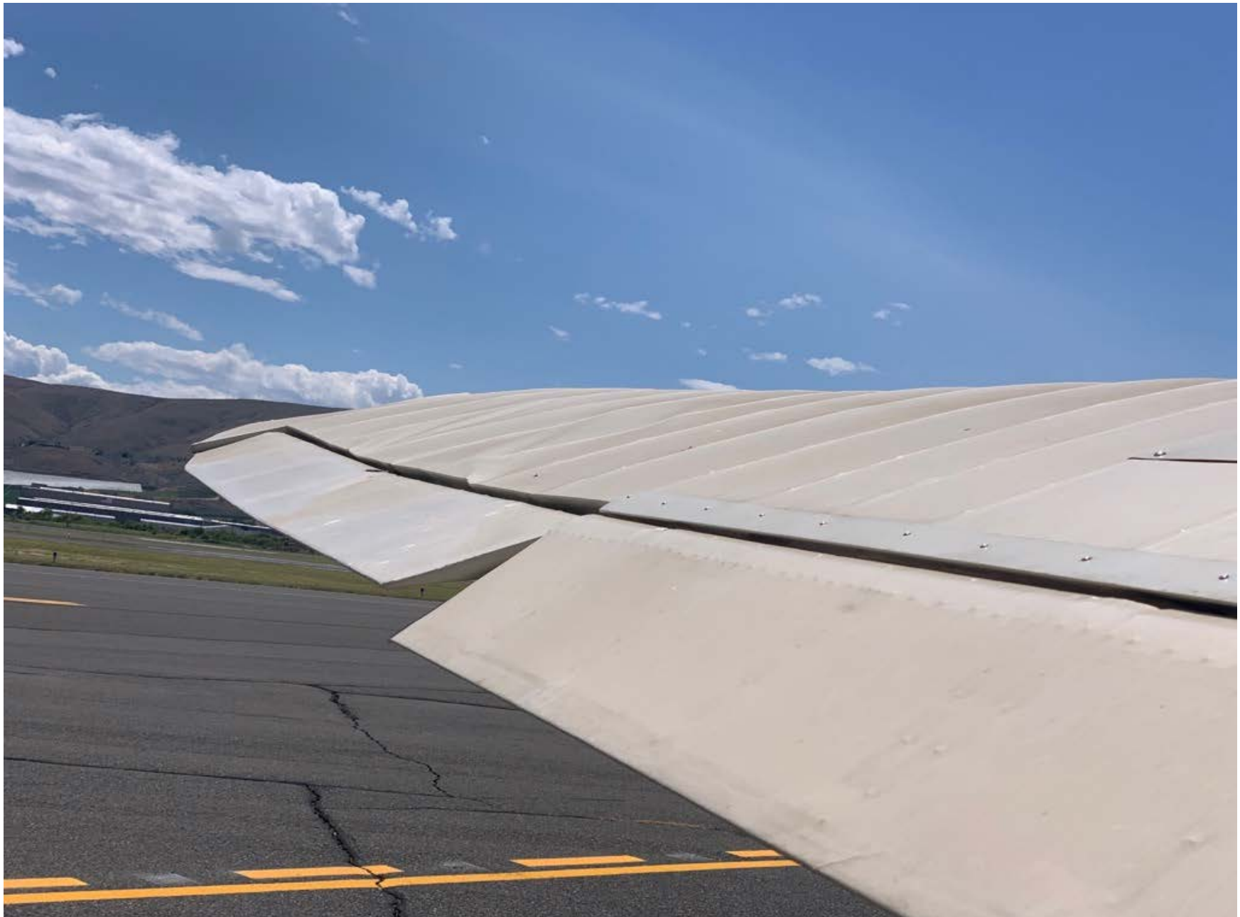
Photo 1 – View of damaged left wing and left aileron (Photo courtesy of the pilot)
