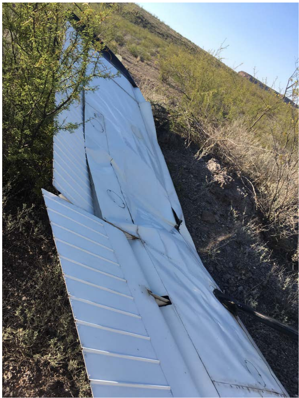
Photo 3 - View of right wing damage (photo courtesy of the pilot)
