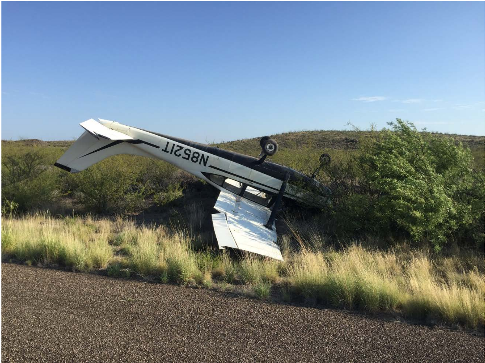
Photo 1 – View of left wing damage (photo courtesy of the pilot)
