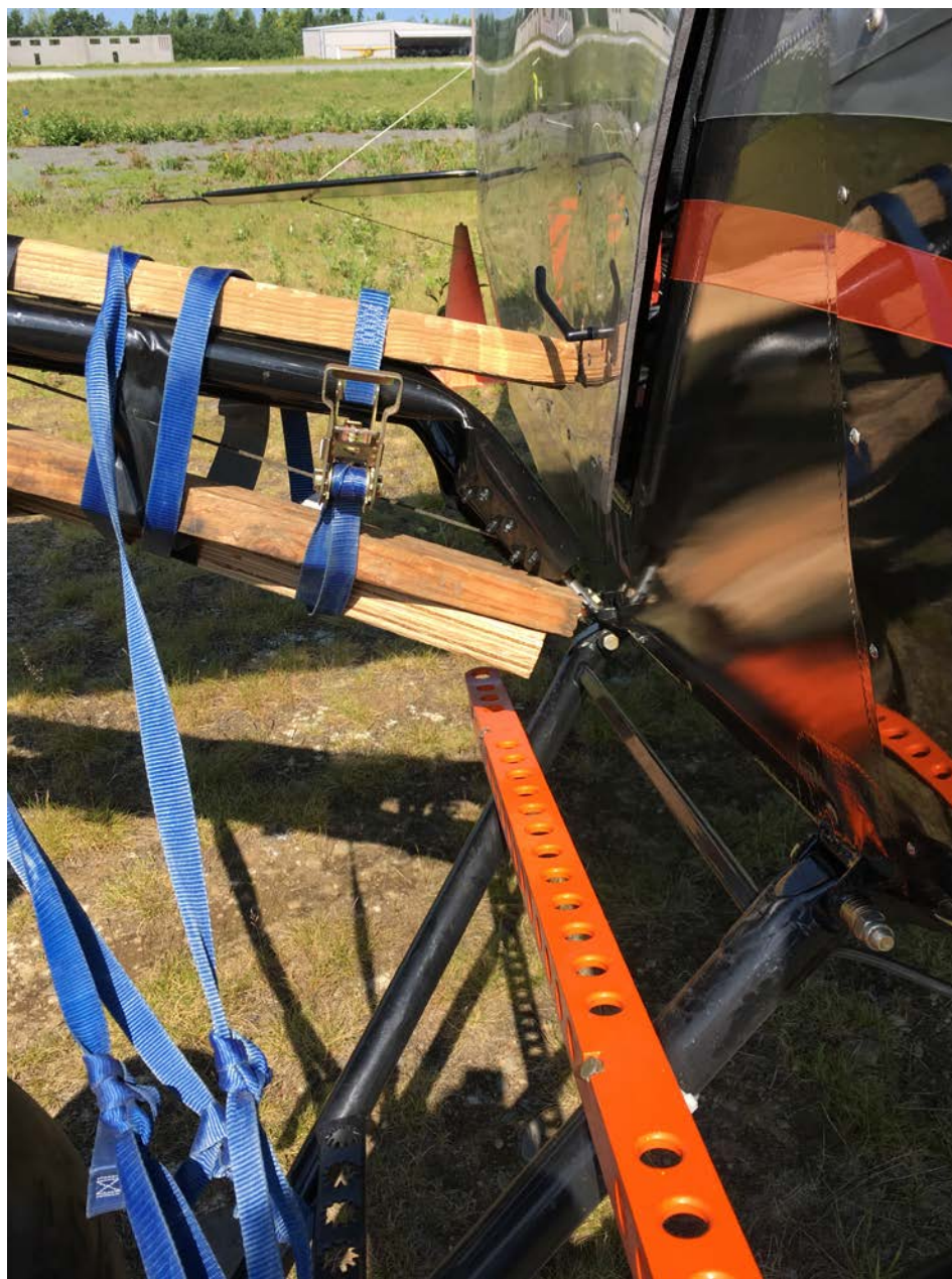
Photo 1 – View of damage to the right wing lift strut (Courtesy of Operator)
