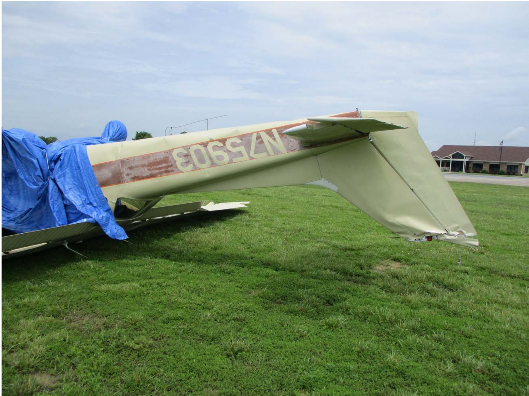
Photo 3 - View of vertical stabilizer damage (photo courtesy of the FAA)
