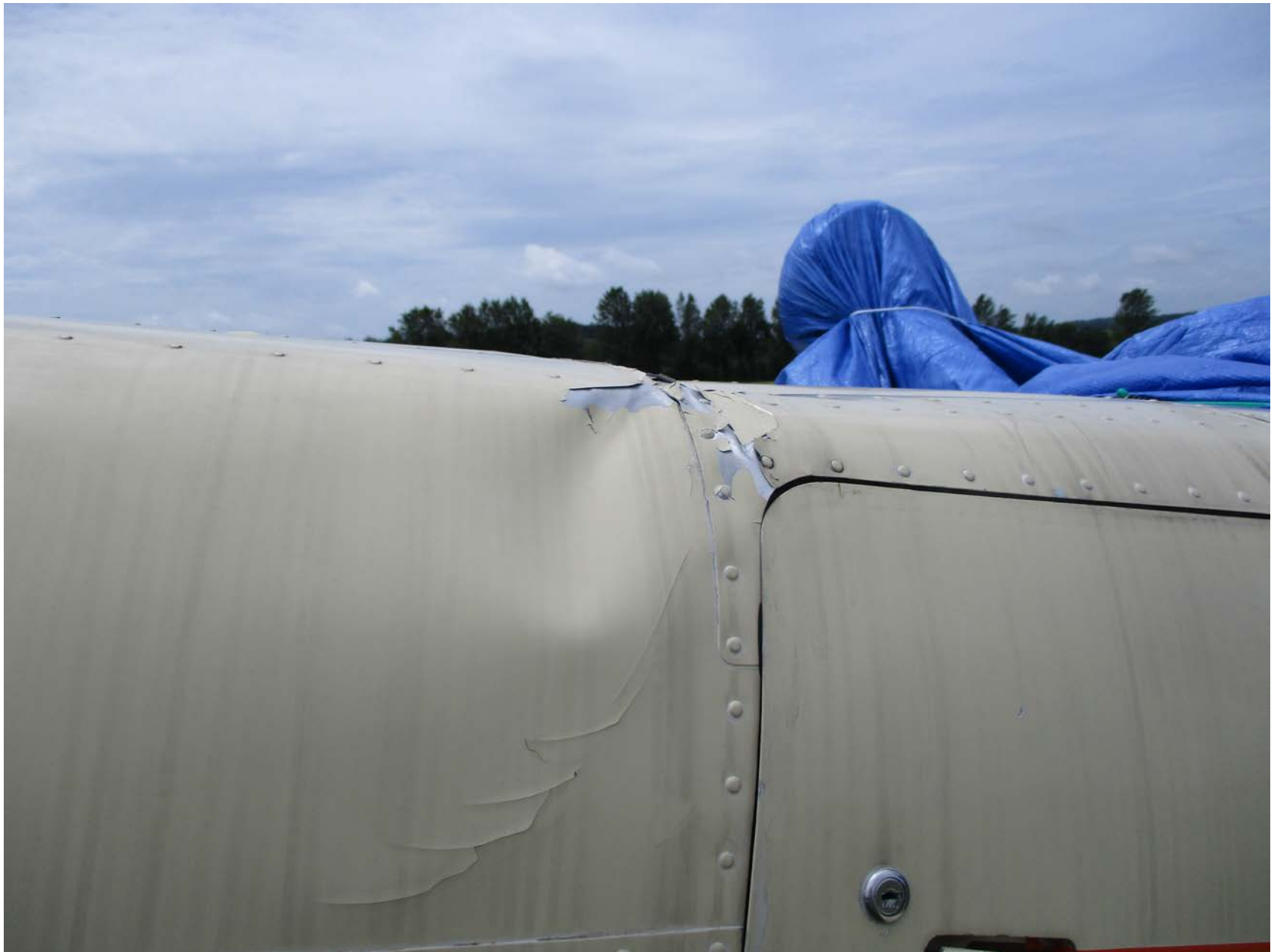
Photo 2 - View of aft fuselage damage (photo courtesy of the FAA)
