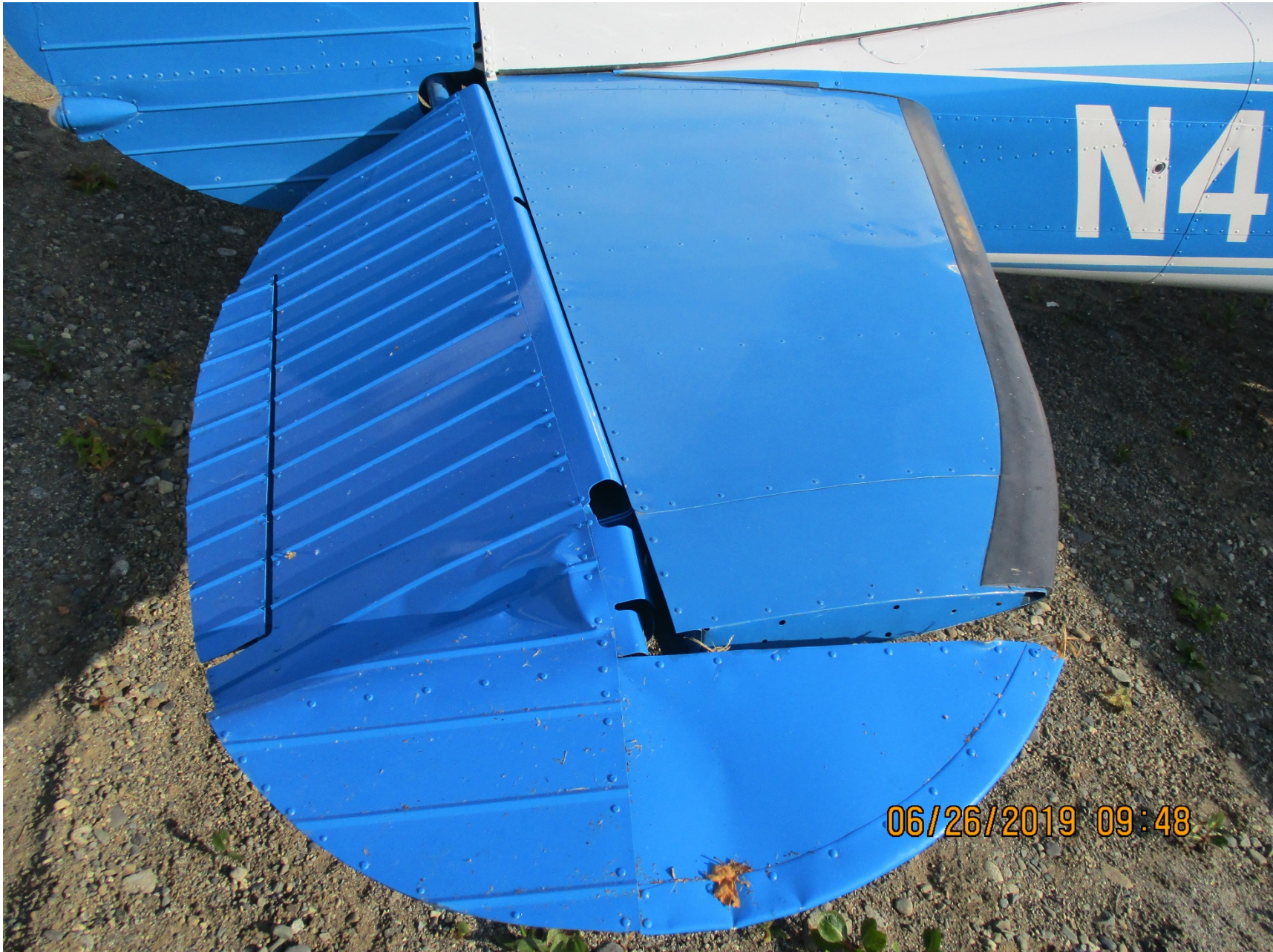
Photo 2 – View of right elevator damage (Photo courtesy of the FAA)
