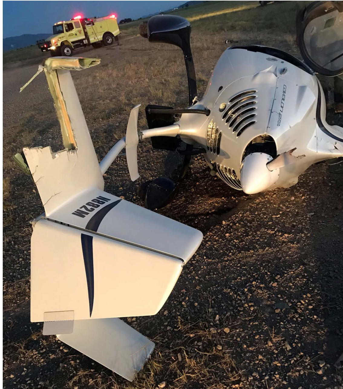
Photo 1 – View of damaged tailboom (Photo courtesy of sheriff's office)
