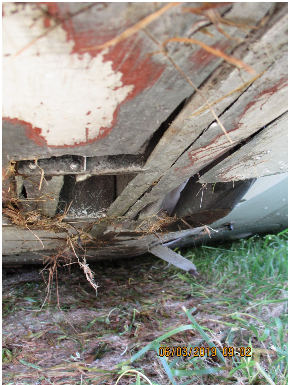
Photo 1 – View of damaged fuselage from underneath (Photo courtesy of the FAA)
