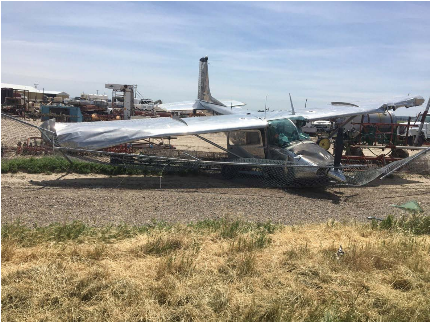
Photo 1 – View of damage to both wings (courtesy of the FAA)
