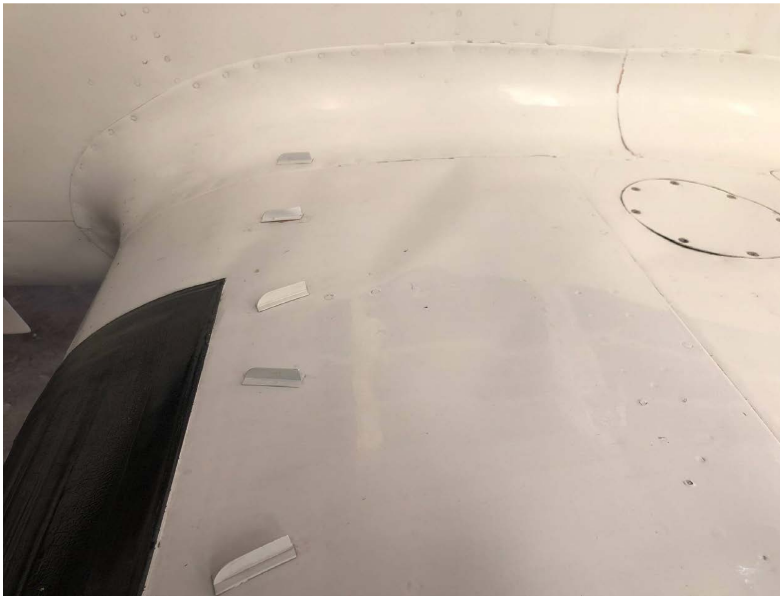
Photo 1 – View of wrinkled left wing (Photo courtesy of the pilot)
