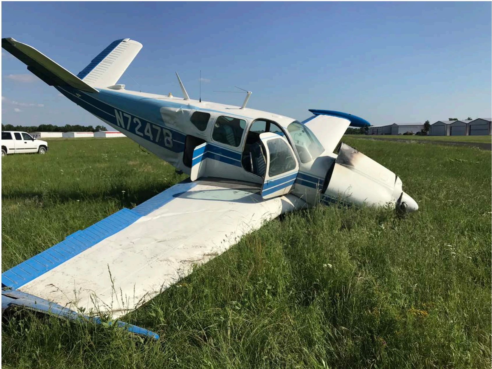
Photo 1 – View of damage to the right wing and the right side of the fuselage (Courtesy of FAA)
