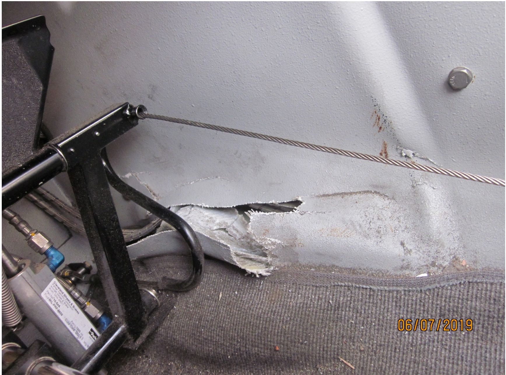
Photo 2 – View of damaged fuselage near left seat right rudder pedals (Photo courtesy of the FAA)
