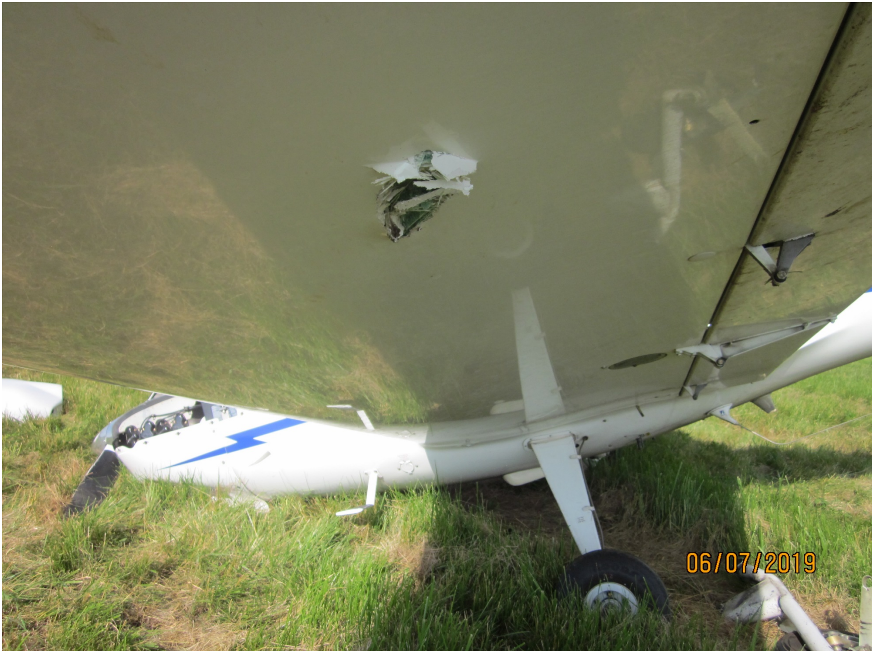
Photo 1 – View of left wing damage from underneath (Photo courtesy of the FAA)
