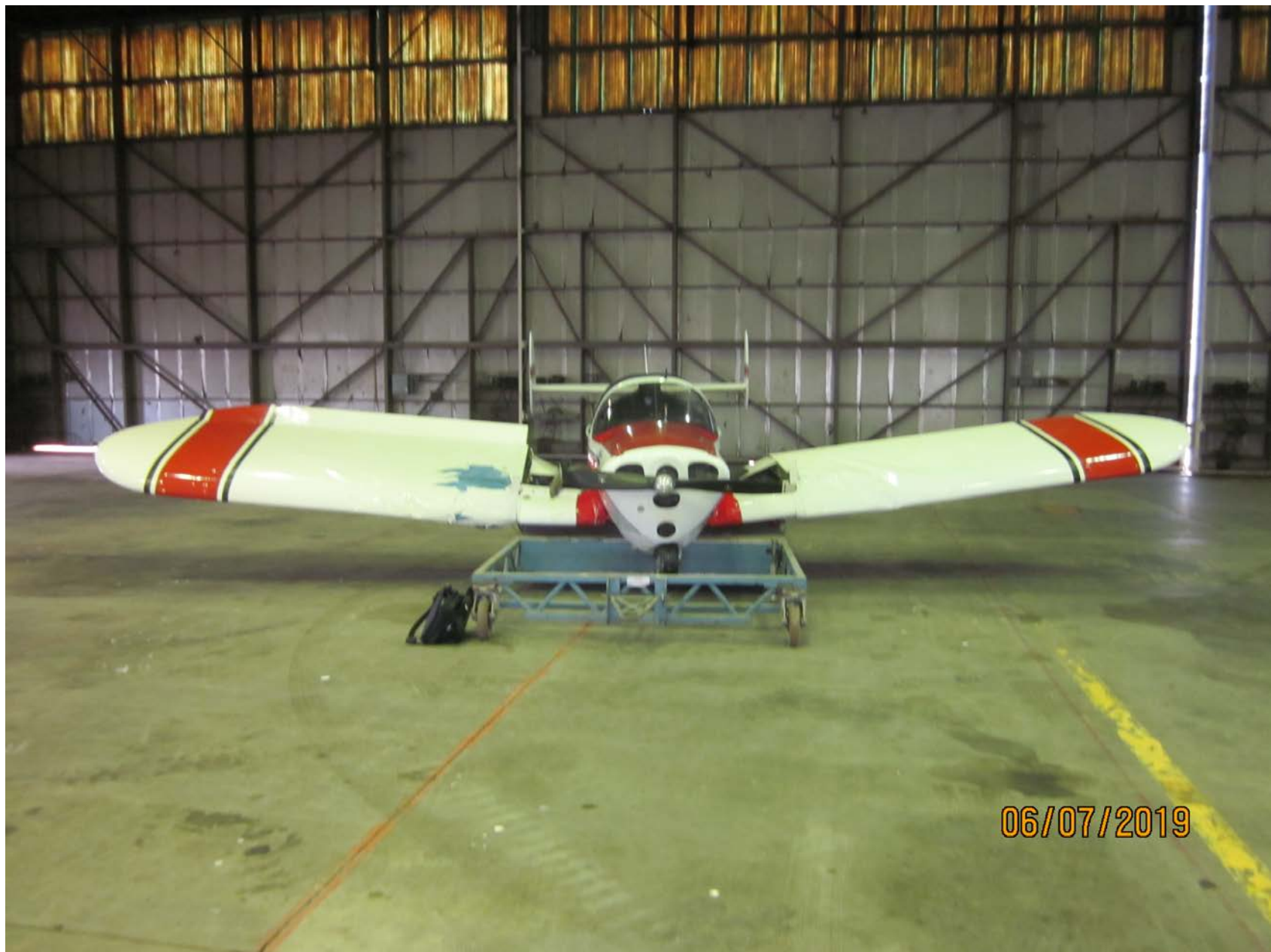
Photo 1 – View of front damage to both wings (photo courtesy of the FAA)
