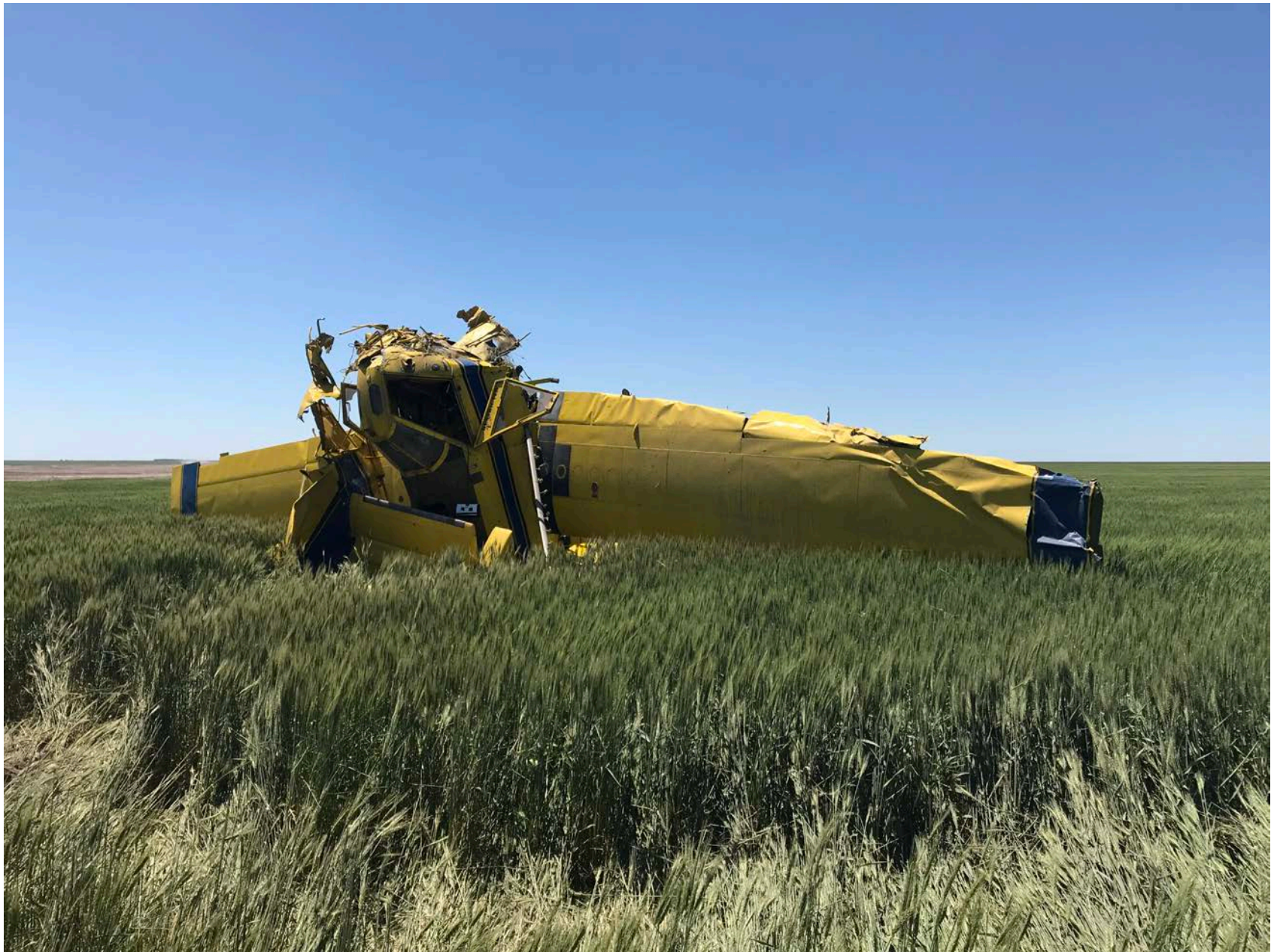
Photo 1 – View of damage to the fuselage and left wing (Courtesy of FAA)
