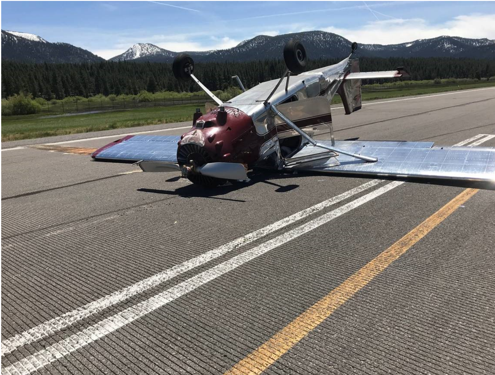
Photo 1 – View of damage to the right wing lift strut and rudder (Courtesy of FAA)
