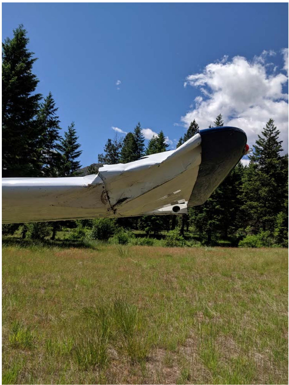
Photo 2 – Close-up view of damaged left wing (courtesy of the FAA)
