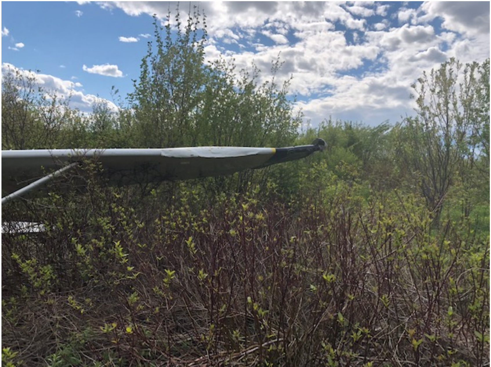
Photo 1 – View of damage to the left wing leading edge (Courtesy of FAA)
