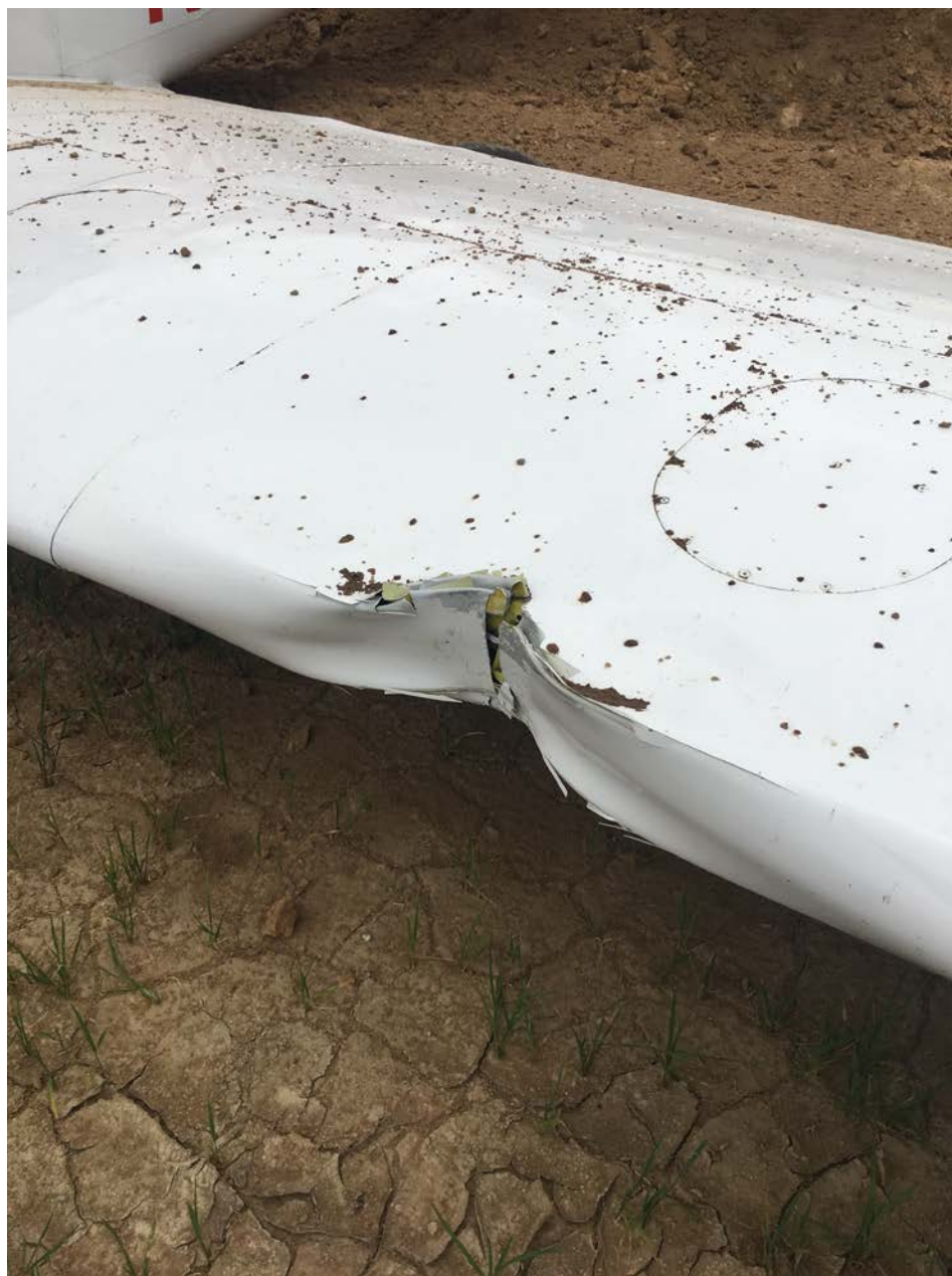
Photo 1 – View of damaged left wing (courtesy of the FAA)
