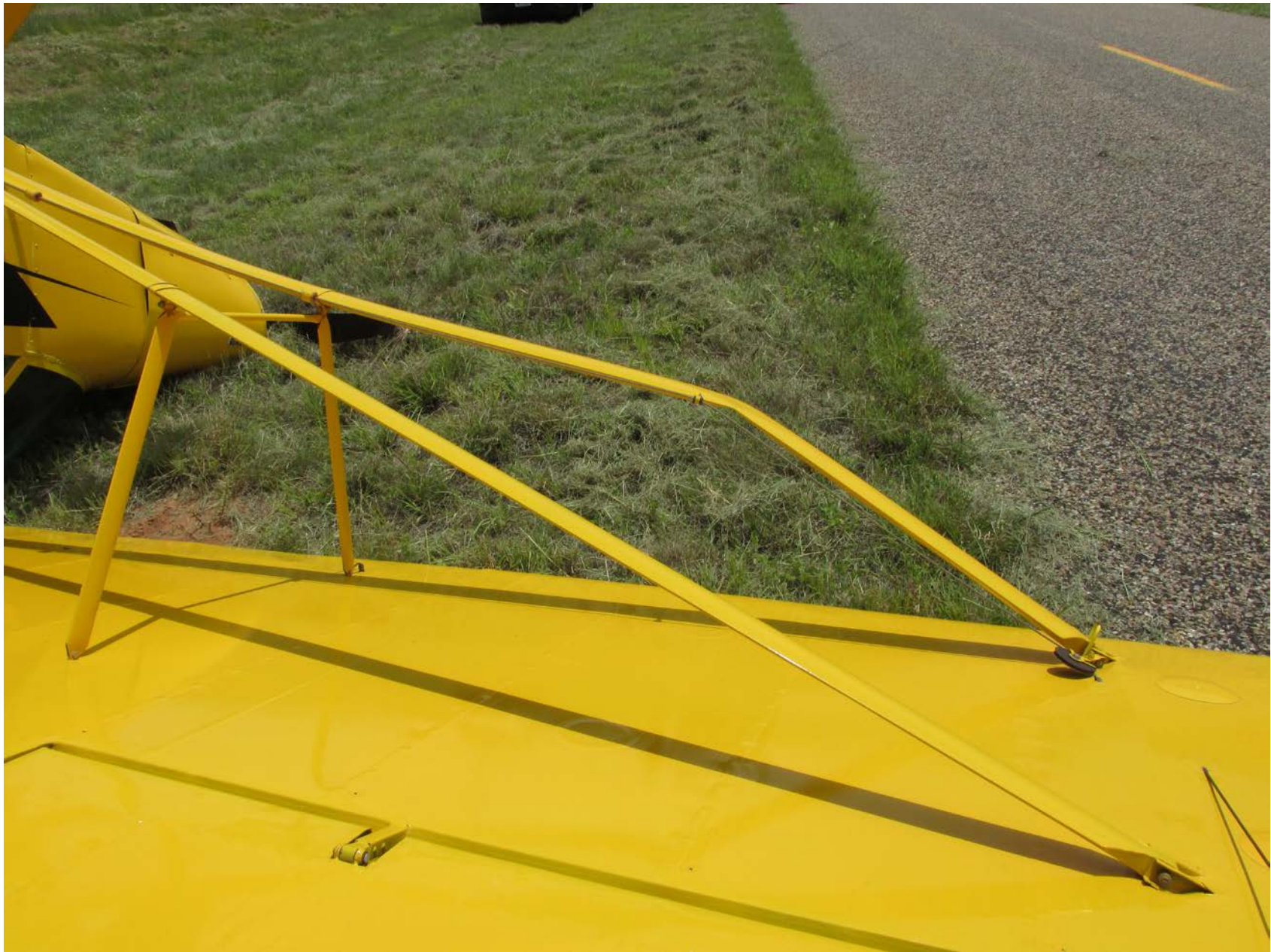
Photo 2 - View of left wing strut damage (photo courtesy of the pilot)
