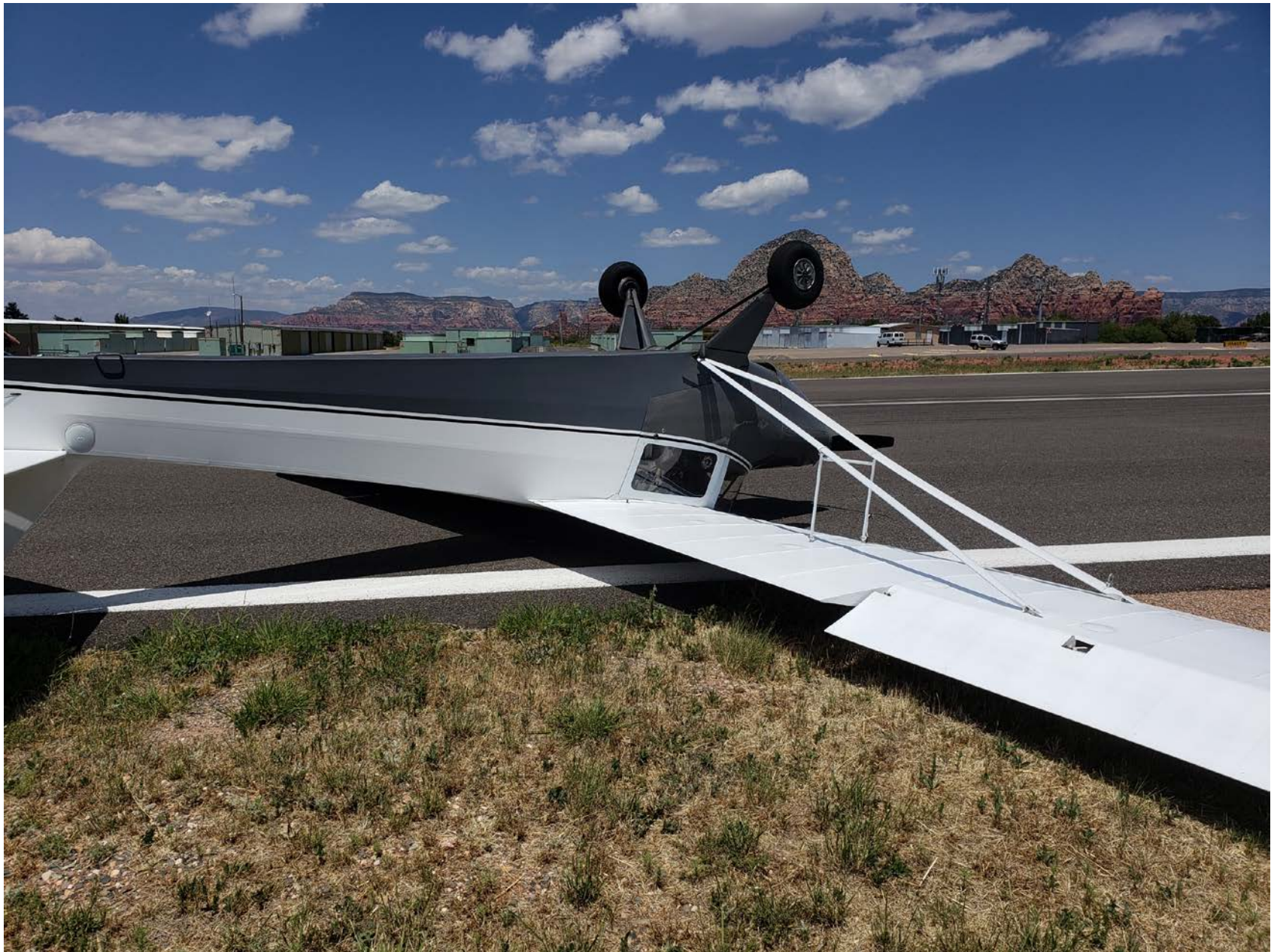
Photo 1 – View of left wing lift strut damage (photo courtesy of the pilot)
