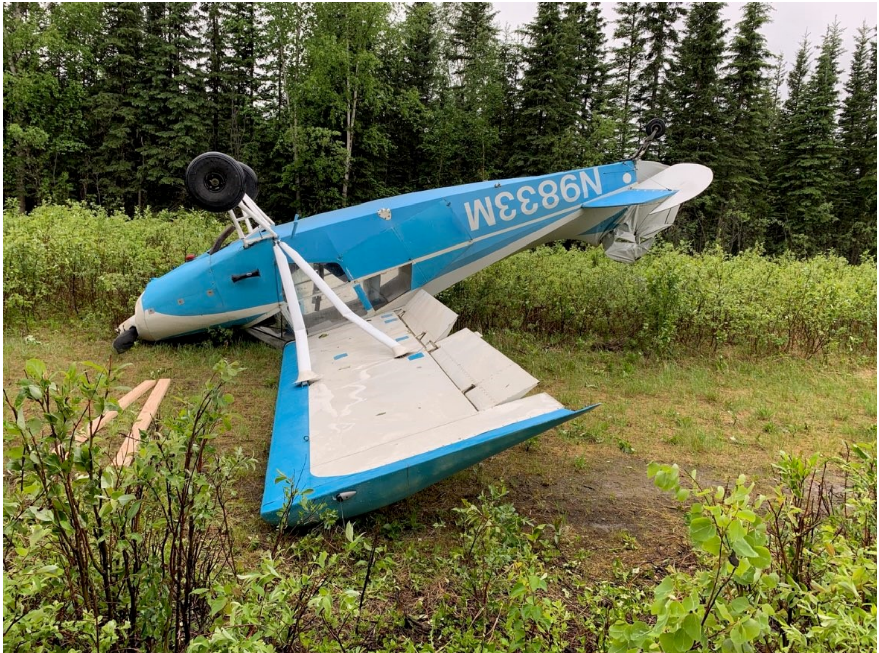
Photo 1 – View of inverted airplane with damaged right wing lift strut and empennage (Photo courtesy unknown)
