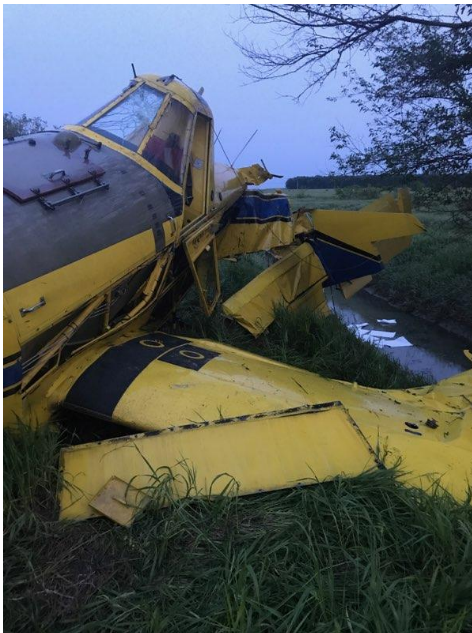
Photo 1 – View of damaged left wing and tailcone (courtesy of the pilot)
