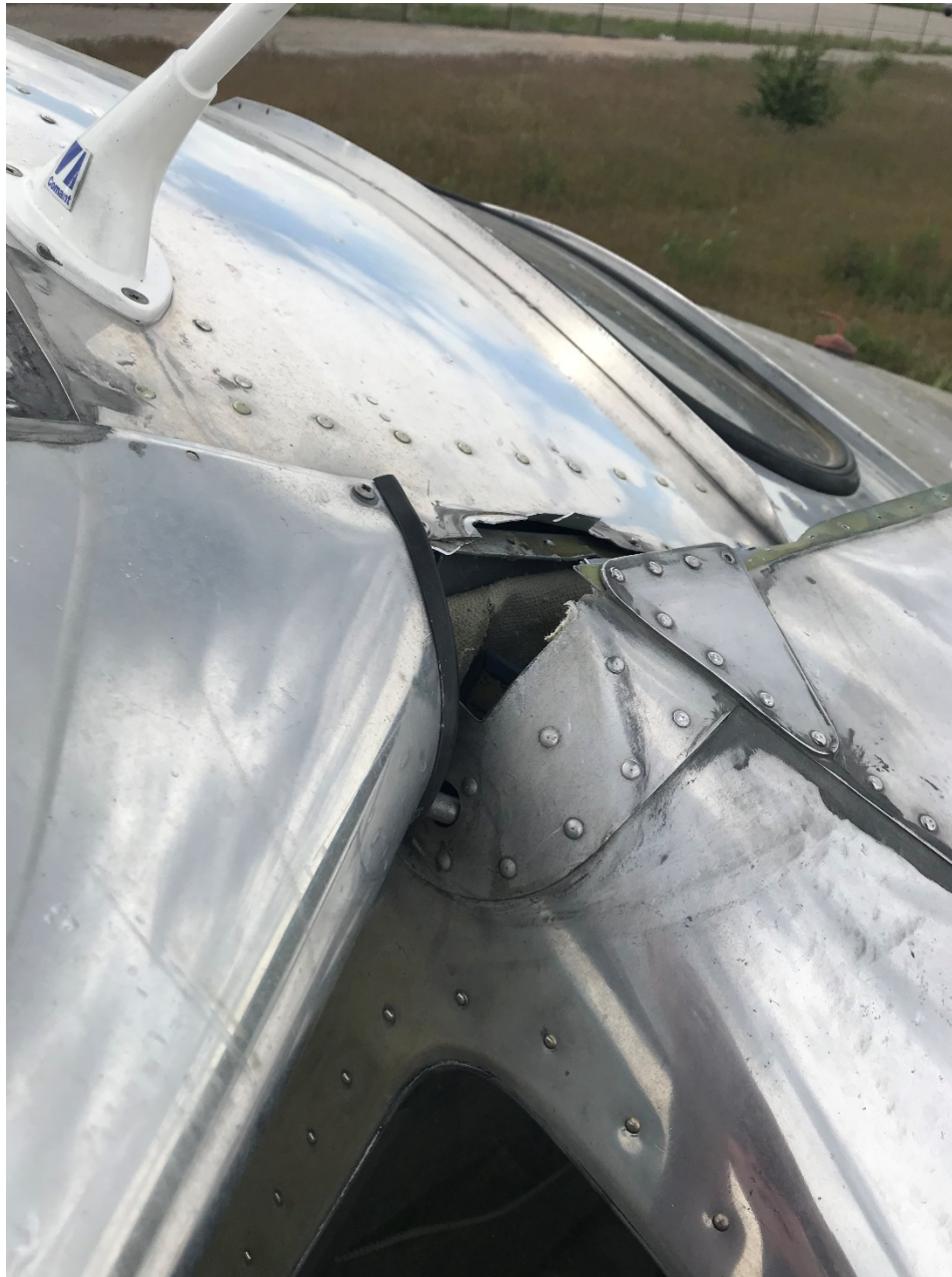
Photo 2 – View of left wing rear attach point to fuselage damage (Photo courtesy of the airport manager)
