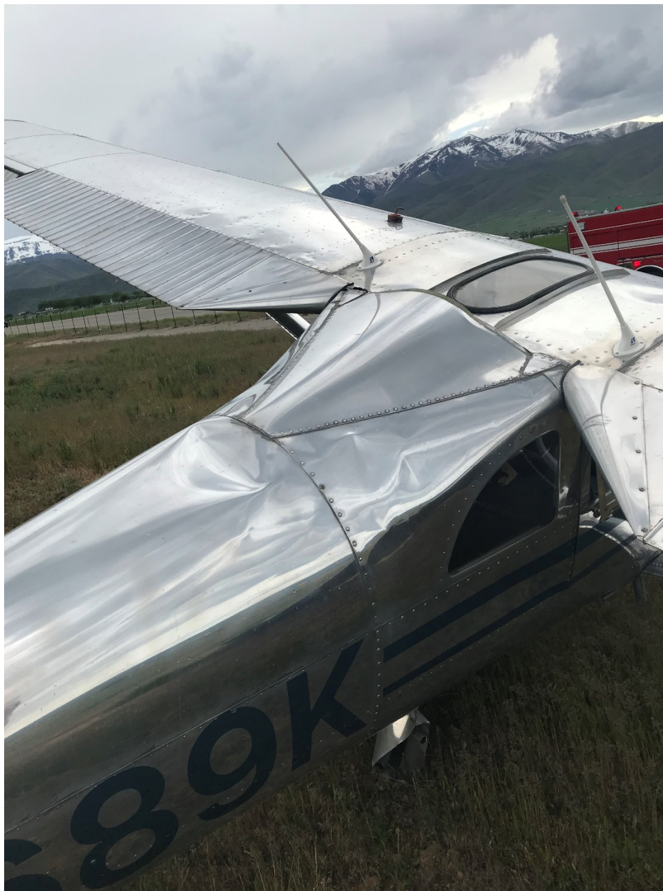
Photo 1 – View of damaged fuselage (Photo courtesy of the airport manager)
