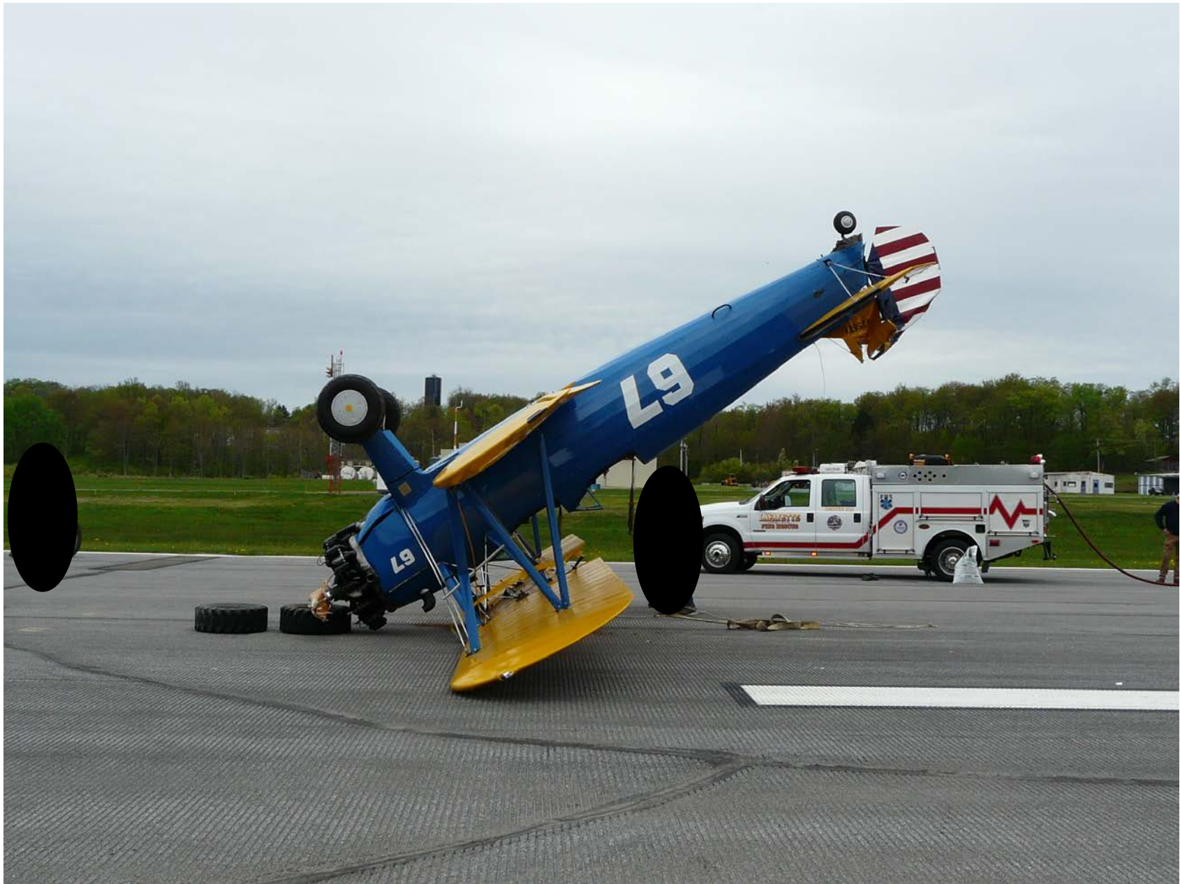
Photo 1 – View of vertical stabilizer damage (photo courtesy of the FAA)
