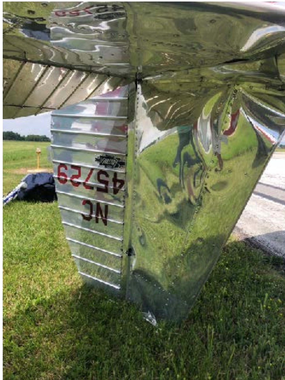
Photo 1 – View of damage to the vertical stabilizer (Courtesy of FAA)
