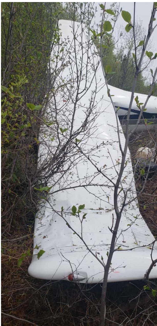
Photo 1 – View of left wing damage (photo courtesy of the FAA)
