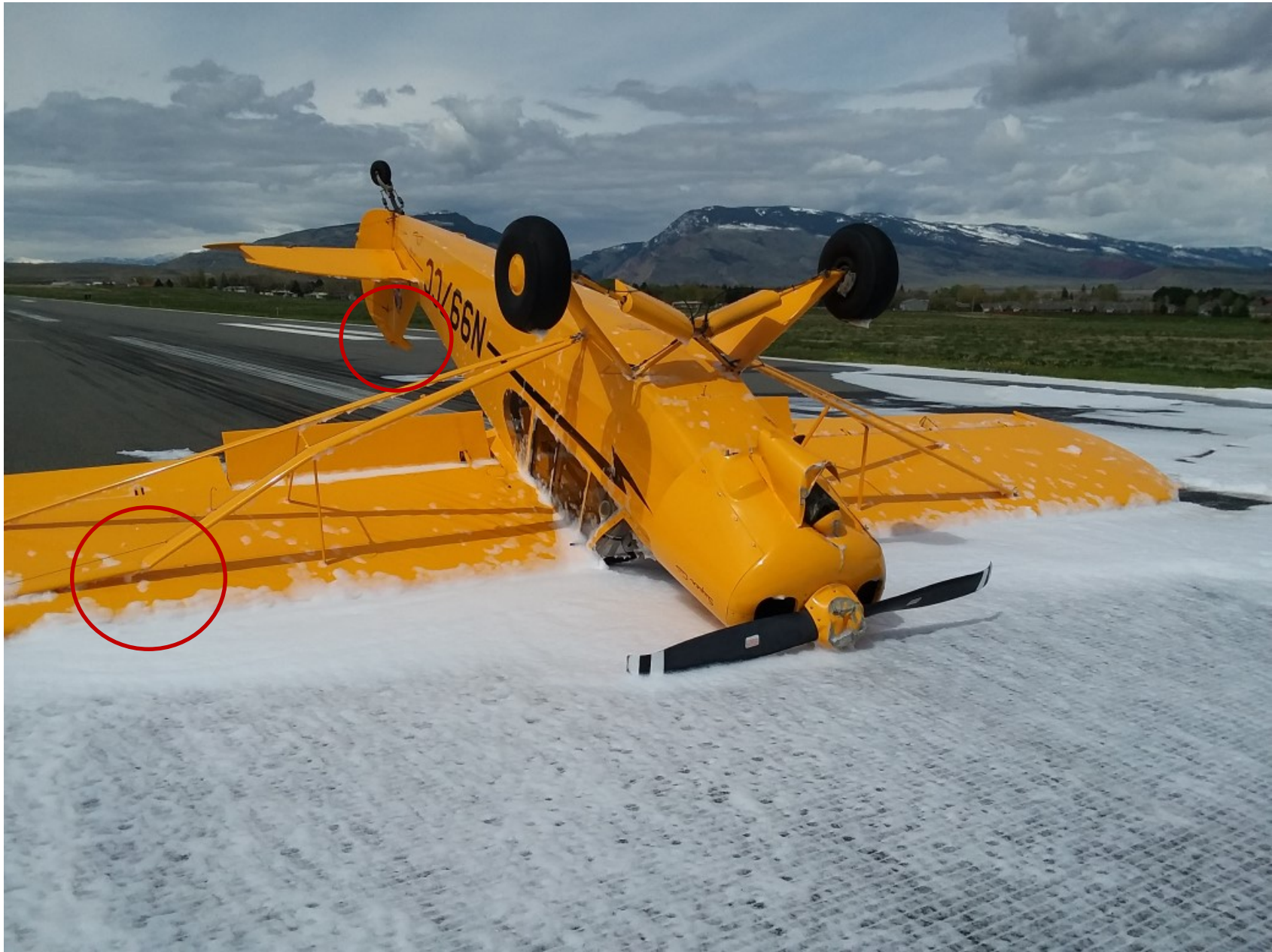
Photo 1 – View of damaged left wing lift strut and rudder (courtesy of the FAA)
