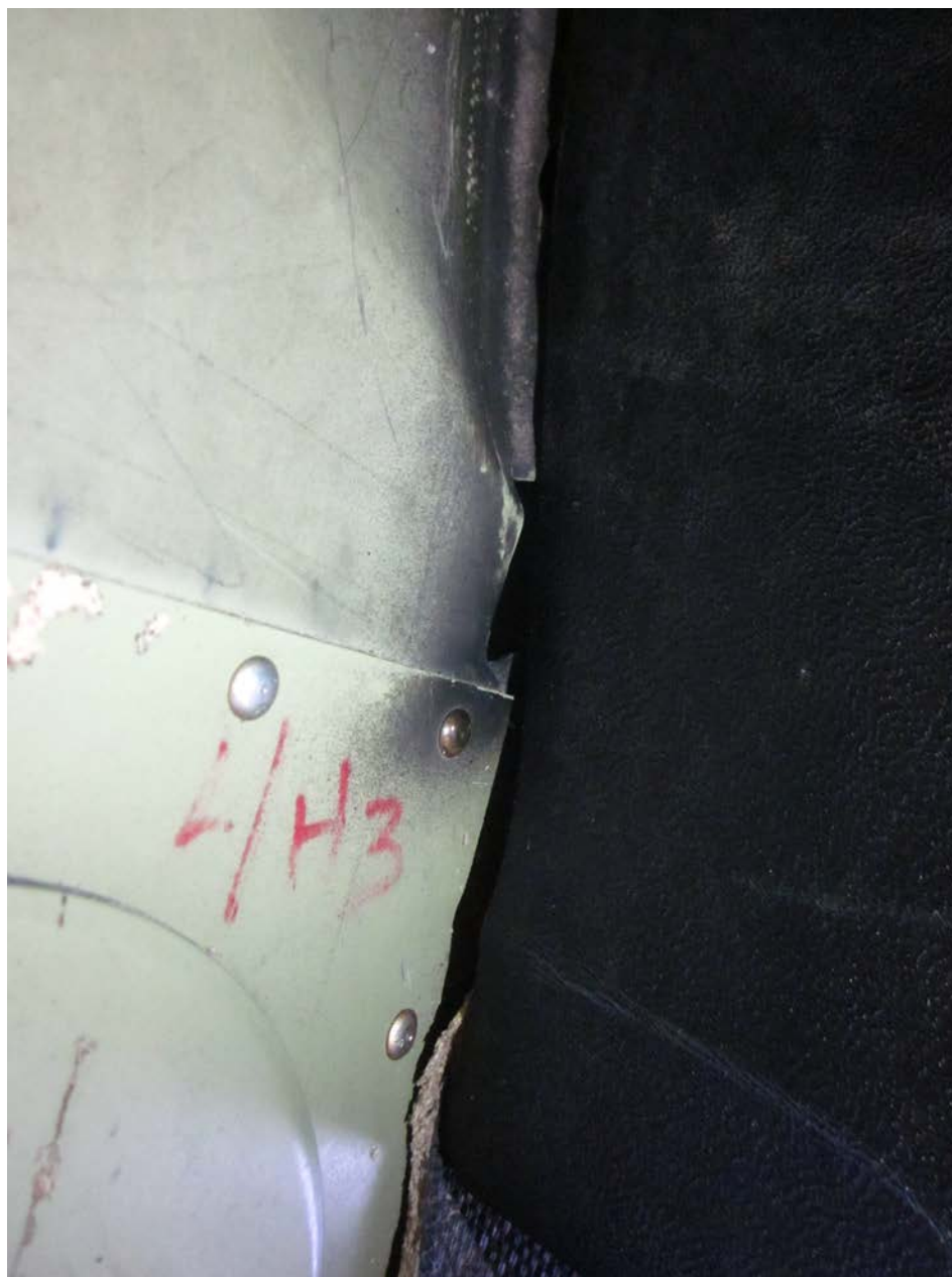
Photo 2 – View of firewall damage (courtesy of the FAA)
