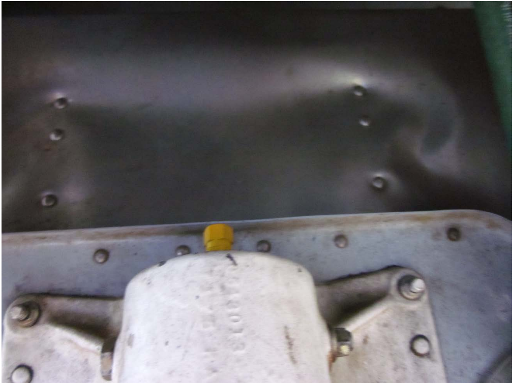
Photo 1 – View of lower fuselage (floor board) damage (courtesy of the FAA)
