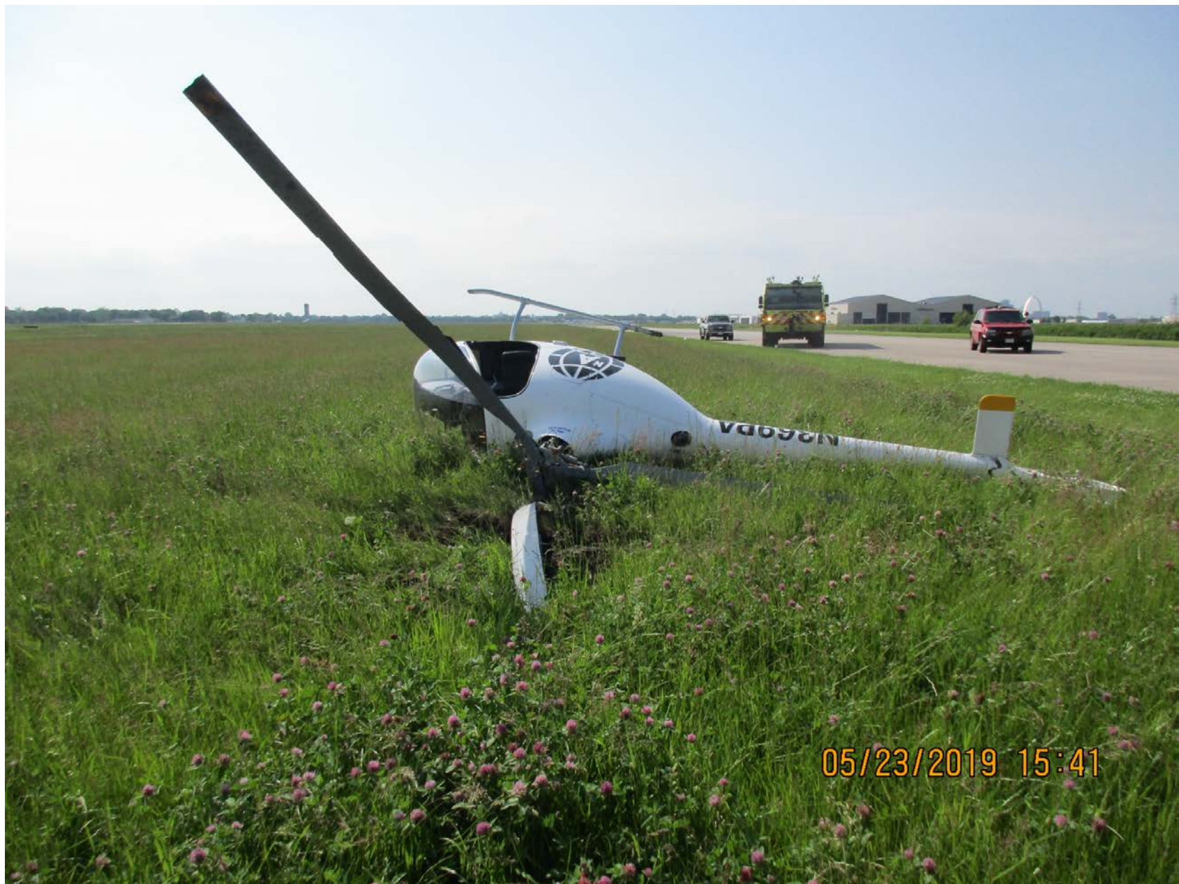
Photo 1 – View of rotor damage (photo courtesy of the FAA)
