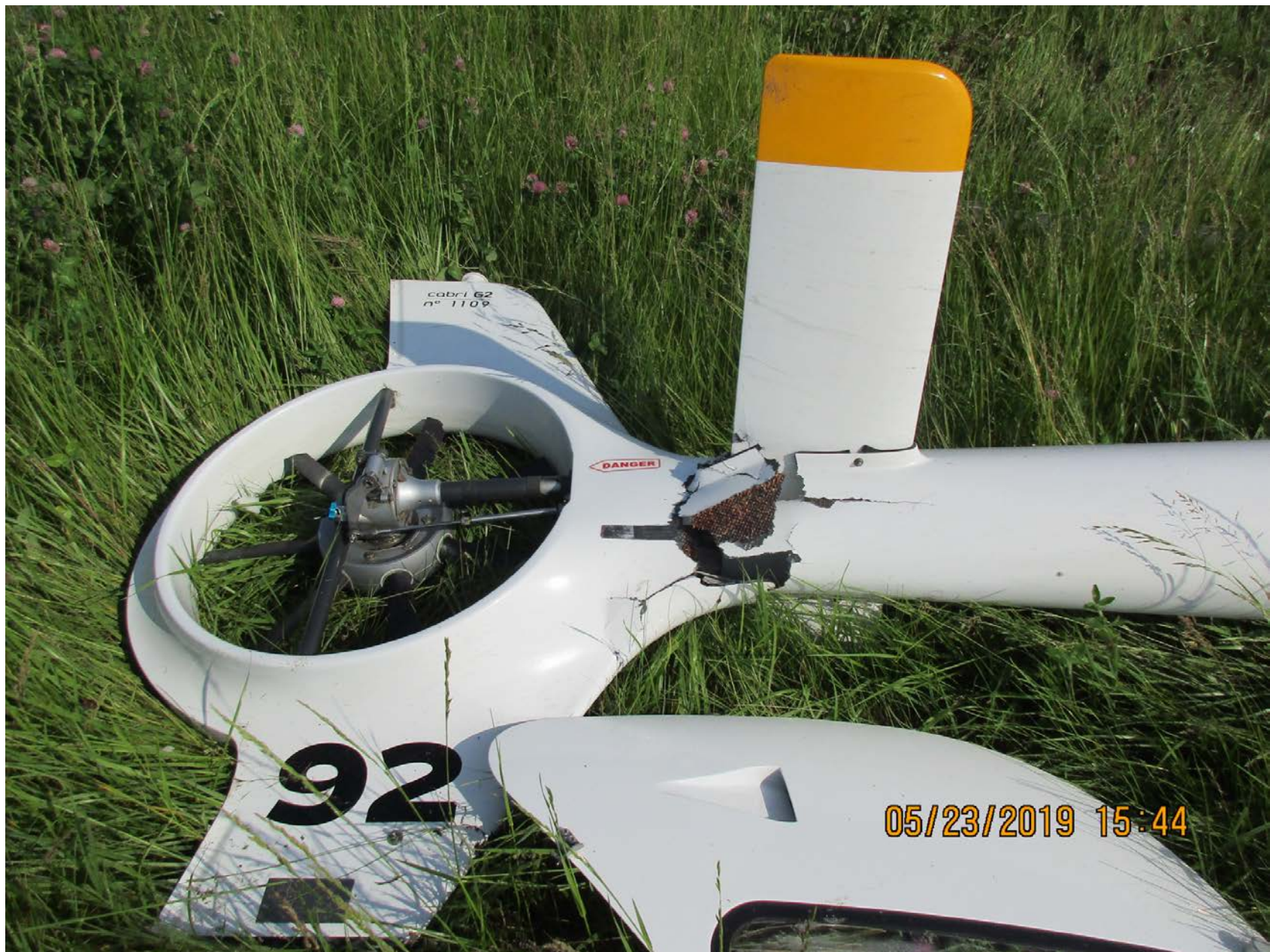
Photo 2 - View of tail boom damage (photo courtesy of the FAA)
