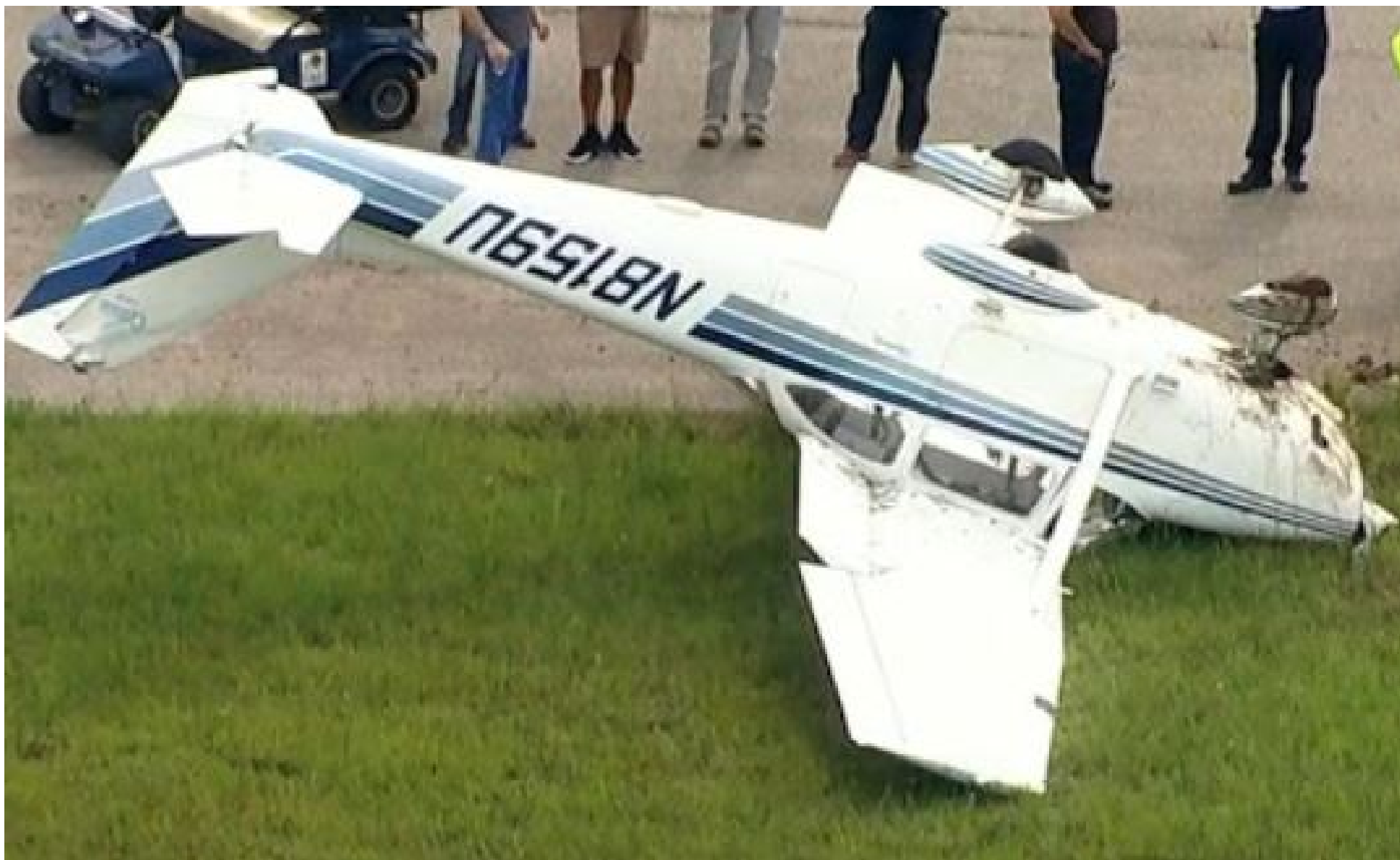
Photo 1 – View of nosed over airplane with damaged rudder (courtesy of the FAA)
