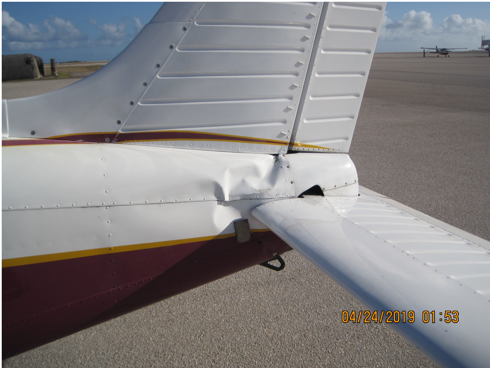
Photo 1 – View of damaged empennage from left side (Photo courtesy of the FAA)
