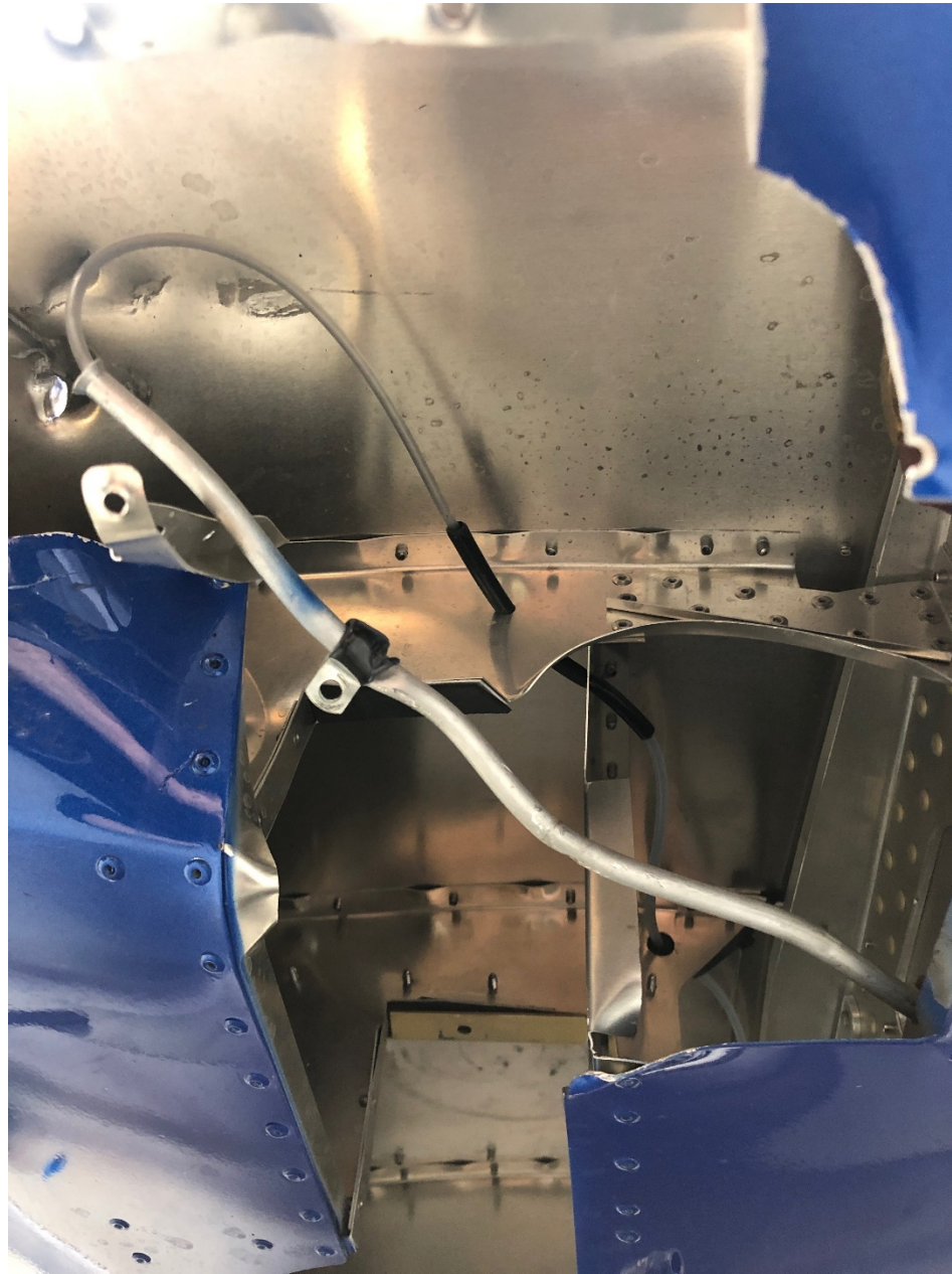
Photo 1 – View of left-wing rib and stringers damage (courtesy of the FAA)
