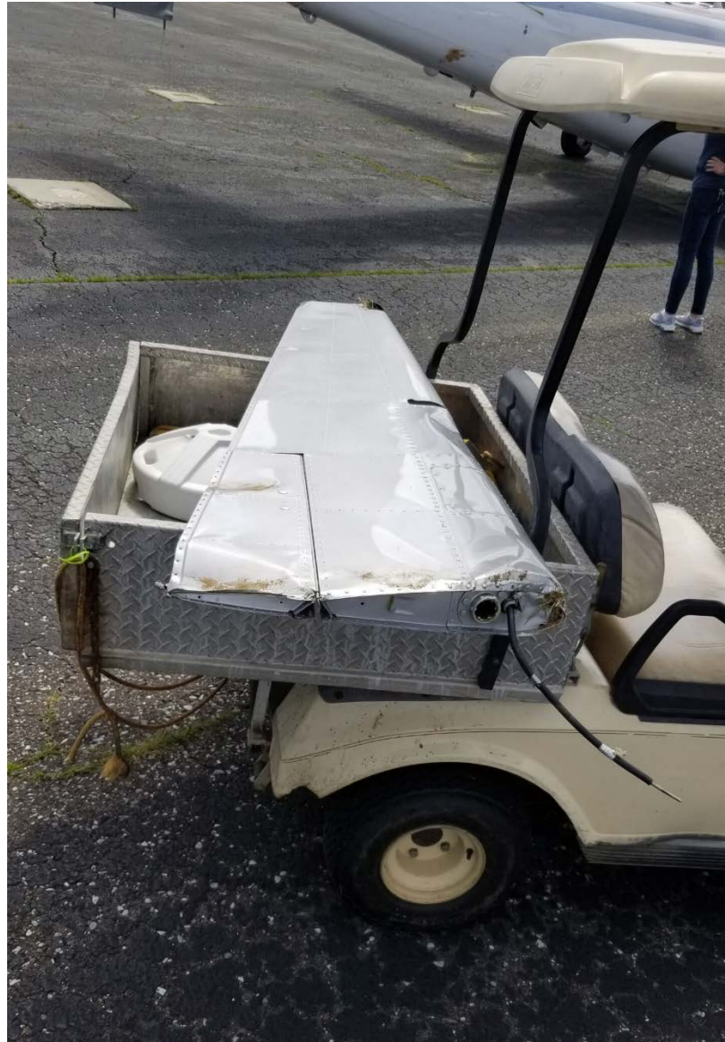
Photo 2 – View of separated right elevator (Photo courtesy of the pilot)
