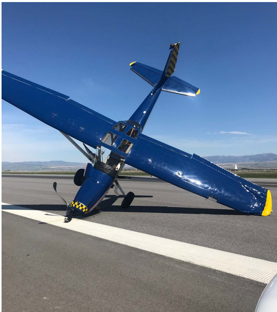
Photo 1 – View of damaged left wing (Photo courtesy of the airport manager)
