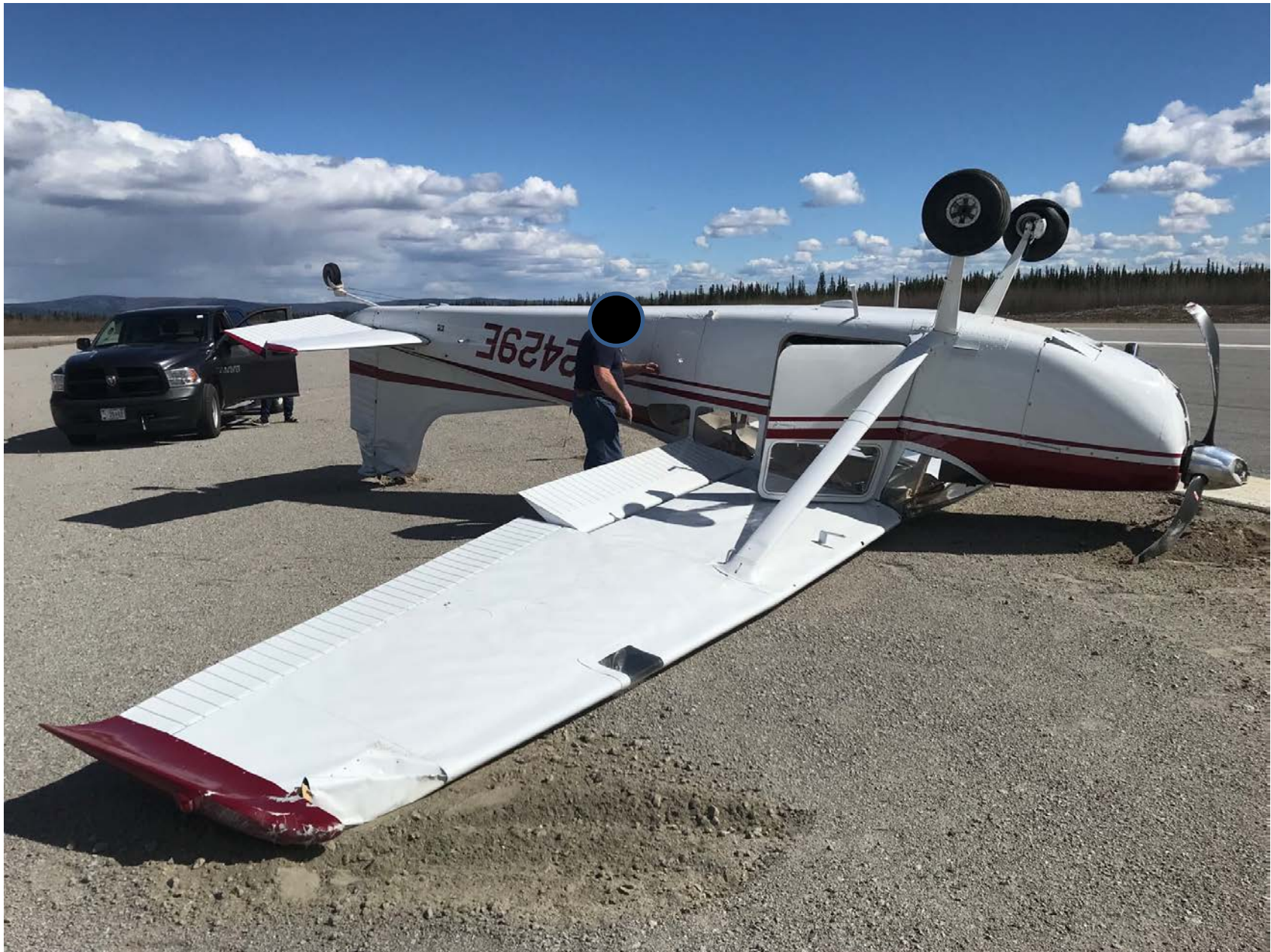
Photo 2 - View of vertical stabilizer and right wing damage (photo courtesy of the FAA)
