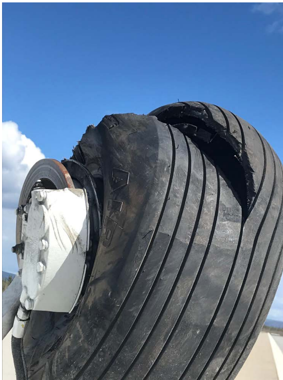
Photo 3 - View of tire damage (photo courtesy of the FAA)
