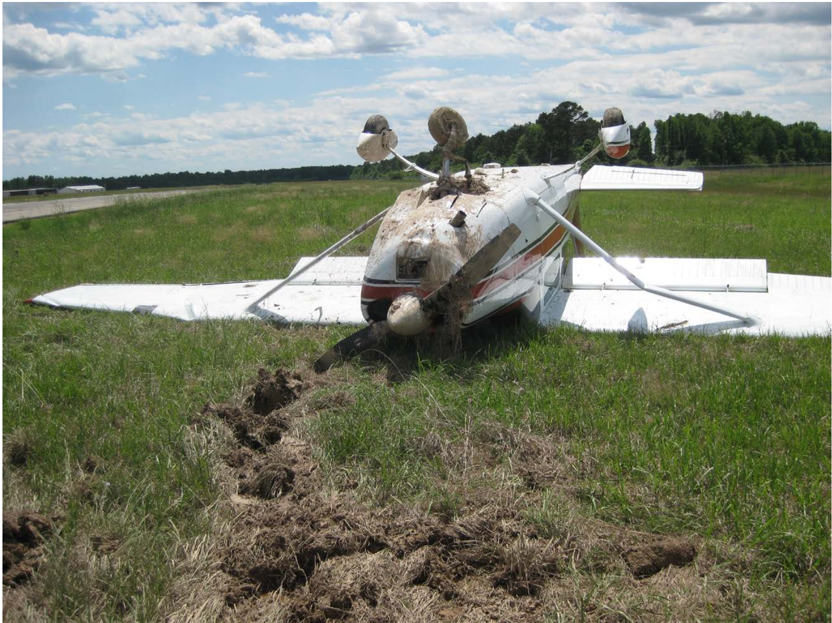
Photo 1 – View of damage to the right wing lift strut (Courtesy of FAA)
