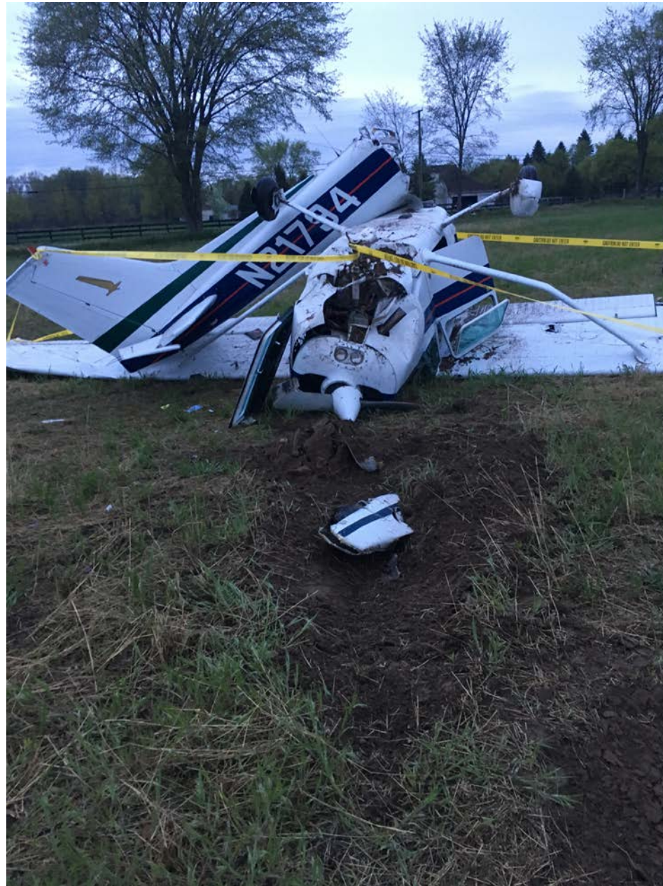
Photo 1 – View of nosed over airplane with damage to both wings and tailcone (courtesy of the FAA)
