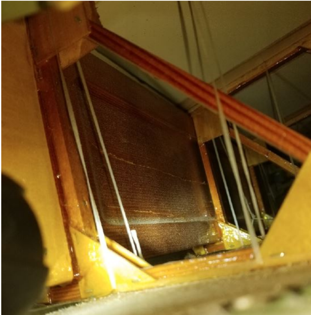
Photo 1 – View of horizontal crack to left lower wing spar (courtesy of the FAA)
