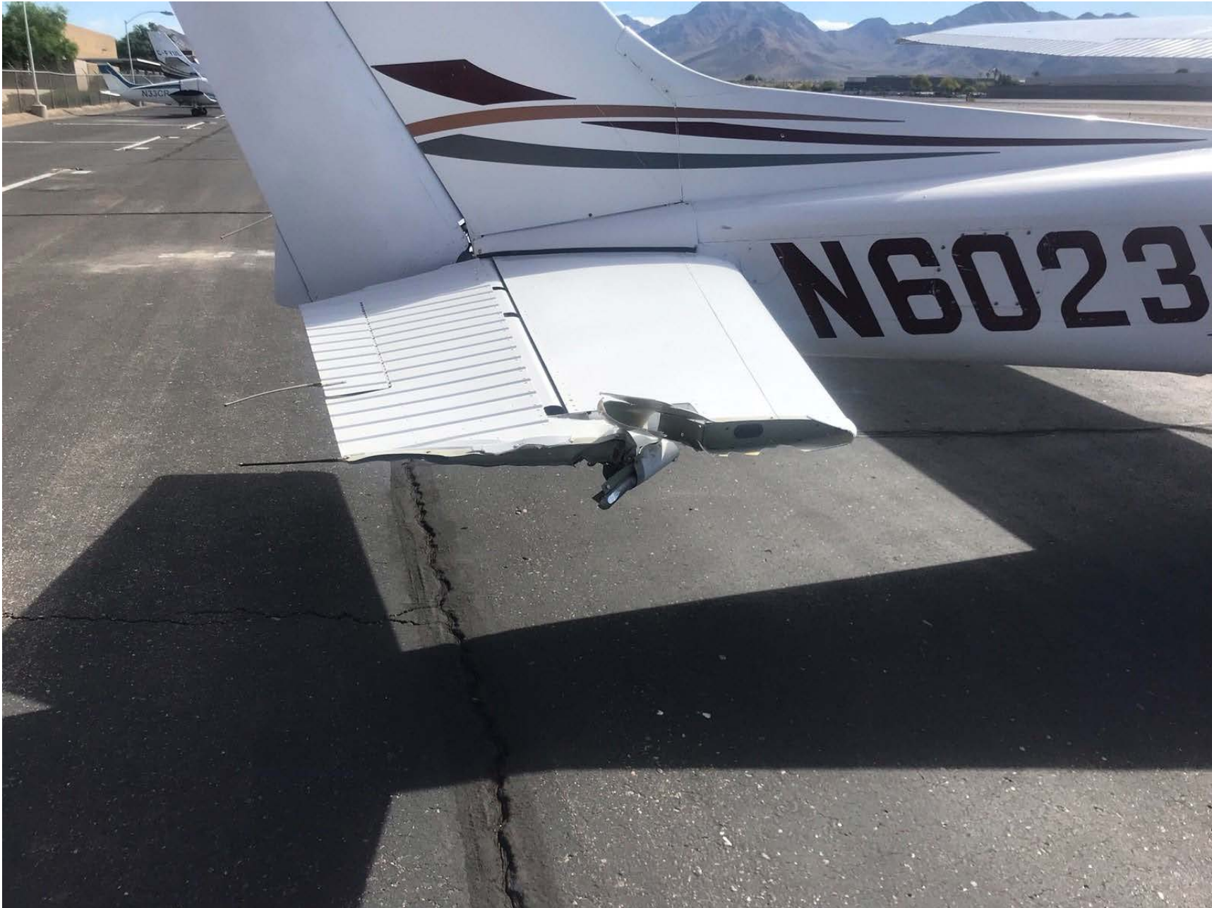
Photo 1 – View of damaged right elevator (Photo courtesy of the operator)
