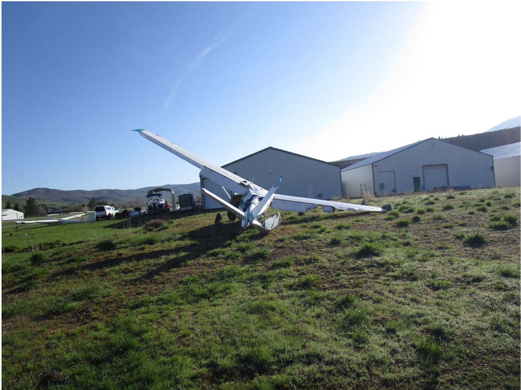
Photo 1 – View of damage to the right horizontal stabilizer, right elevator and right wing (Courtesy of FAA)
